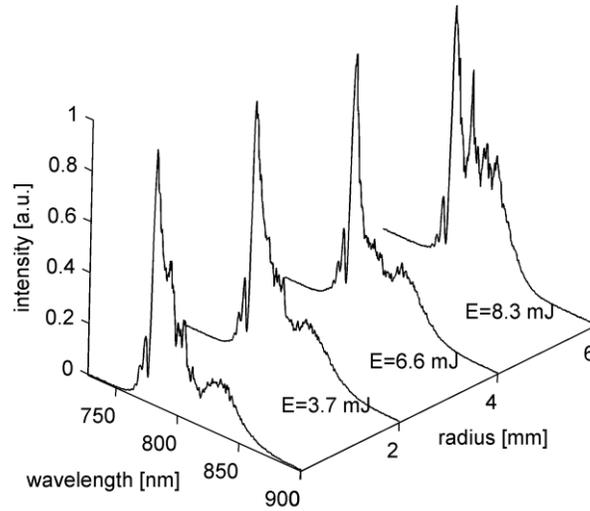
Fig. 3 Spectra measured behind 1 mm pinhole placed at different positions along the non-guided axis of the beam (the position  $0$  is the beam center). The pulse energies contained within the radii are also indicated.
