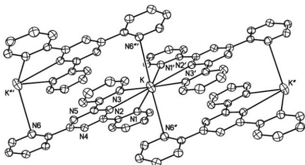
**Fig. 1** View of the 1D structure of **1**. The H atoms have been omitted. Displacement ellipsoids are drawn at the 40% probability level. Symmetry codes: ' = 2 - x, y, 3/2 - z; '' = x, 2 - y, z + 1/2; ''' = 2 - x, 2 - y, 1 - z. Selected bond lengths (Å) and angles (°): K–N1 2.946(2), K–N2 2.942(2), K–N3 2.902(2), K–N6'' 3.311(2); N1–K–N2 55.94(6), N2–K–N3 56.73(6), N1–K–N6'' 80.50(6), N2–K–N6'' 77.87(6), N3–K–N6'' 80.64(6), N6''–K–N6''' 143.22(8).
