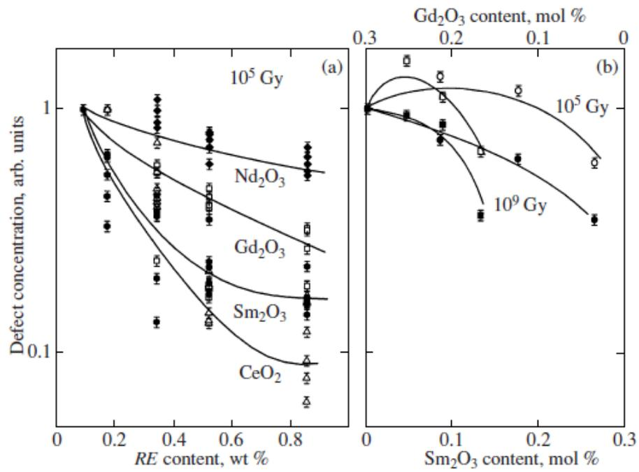
Fig. 3. Defect concentration as a function (a) of the content of different *RE* for all irradiation doses and (b) of *Sm* content for doses of  $10^5$  and  $10^9$  Gy. The lines are guide for the eye only.
