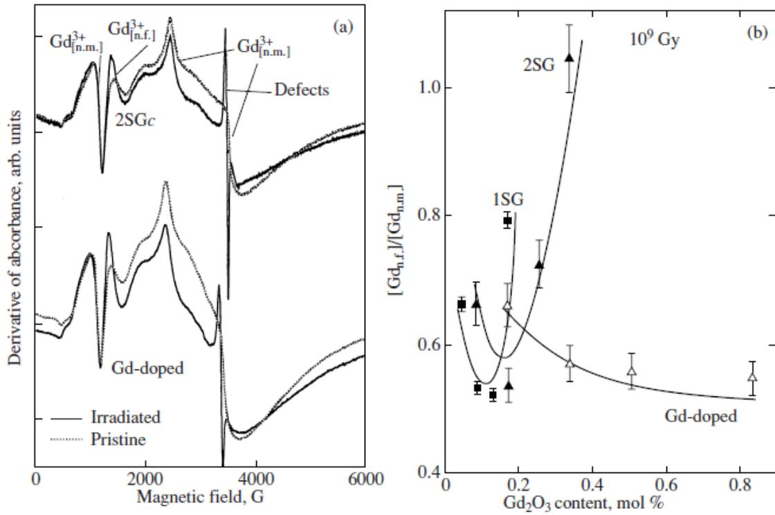
**Fig. 1.** (a) EPR spectra of 0.34 mol % codoped (*RE* oxide amounts with a Sm/Gd ratio of 3: 1 (2SGc)) and Gd-doped aluminoborosilicate glasses. (b) Relative amount of  $Gd^{3+}$  ions located in network former positions as a function of  $Gd_2O_3$  concentration for codoped and singly doped glasses (the lines are guide to the eye only).
