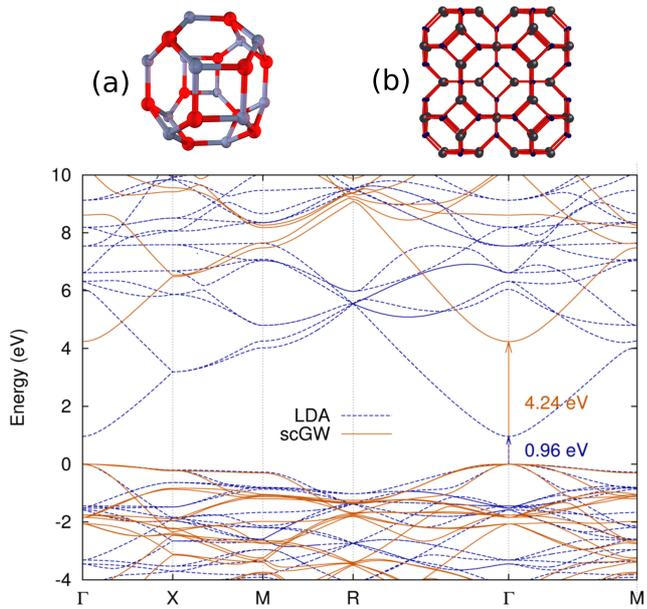
FIG. 1: Band structure of ZnO sodalite structure in DFT-LDA and sc-GW. The gap is direct at  $\Gamma$  and estimated to be 4.2 eV in sc-GW and 0.9 eV in LDA. The inset (a) presents an elementary cage of the sodalite illustrated in inset (b).
