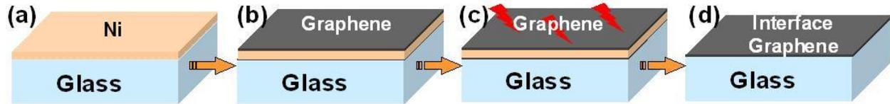
Figure 1. Schematic of interfacial graphene growth: (a) Ni evaporation on glass, (b) dc-PECVD at 450 °C, (c) etching of the surface graphene by H<sub>2</sub>O plasma, followed by wet Ni etching, (d) final graphene-on-glass sample.
