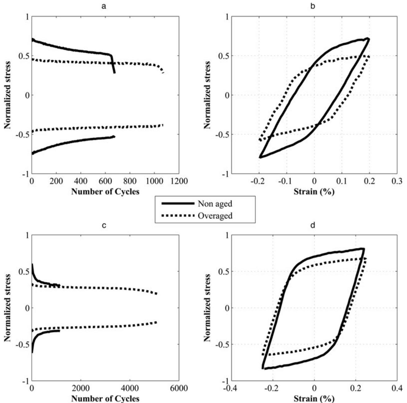
**Fig. 3** LCF tests at 250°C (a) Axial stress cyclic evolution versus number of cycles: aged and non-aged LFC-A319; (b) Stabilized hysteresis loop: aged and non-aged LFC-A319; (c) Axial stress cyclic evolution versus number of cycles: aged and non-aged LFC-A356; (d) Stabilized hysteresis loop: aged and non-aged LFC-A356.
