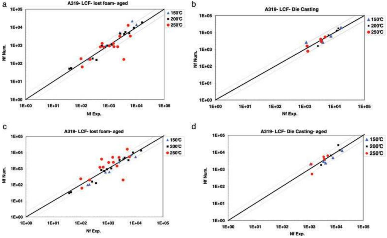
**Fig. 8** Experimental fatigue life versus predicted fatigue life: (a)  $W_{\sigma_{\max}}$  criterion for A319-LFC, (b)  $W_{\sigma_{\max}}$  criterion for A319-DC, (c)  $W_{\Delta\sigma}$  criterion for A319-LFC, (d)  $W_{\Delta\sigma}$  criterion for A319-DC.
