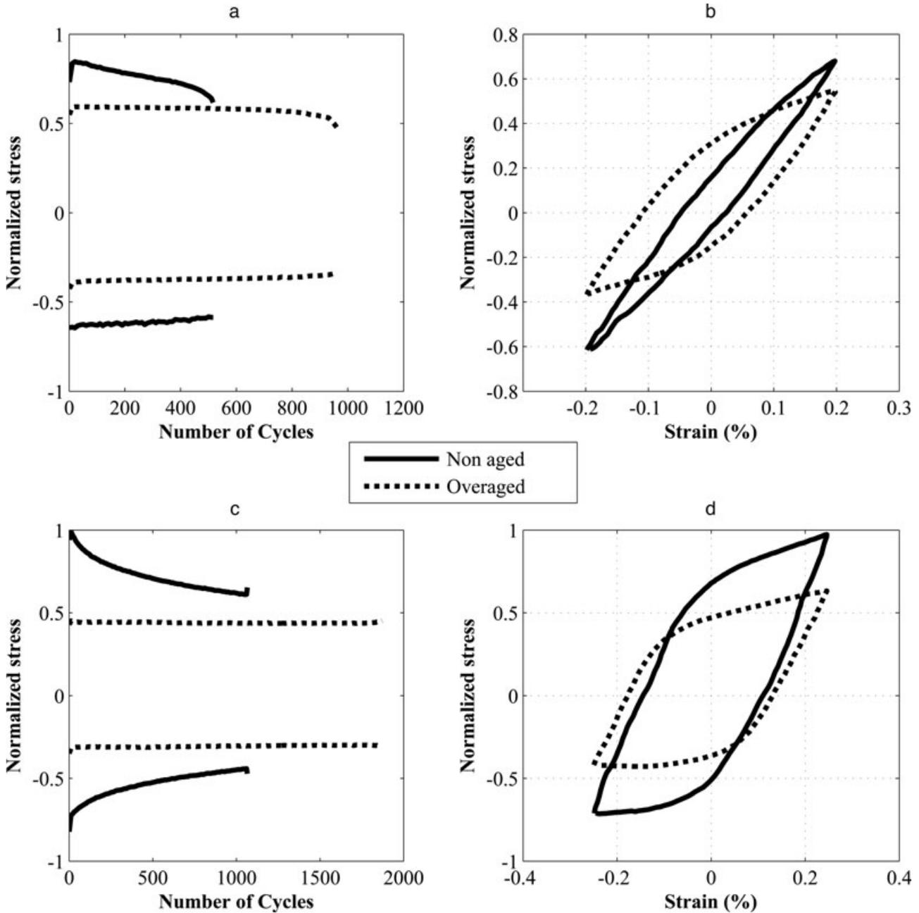
**Fig. 4** TMF tests between 100°C and 250°C (a) Axial stress cyclic evolution versus number of cycles: aged and non-aged LFC-A319; (b) Stabilized hysteresis loop: aged and non-aged LFC-A319; (c) Axial stress cyclic evolution versus number of cycles: aged and non-aged LFC-A356; (d) Stabilized hysteresis loop: aged and non-aged LFC-A356.
