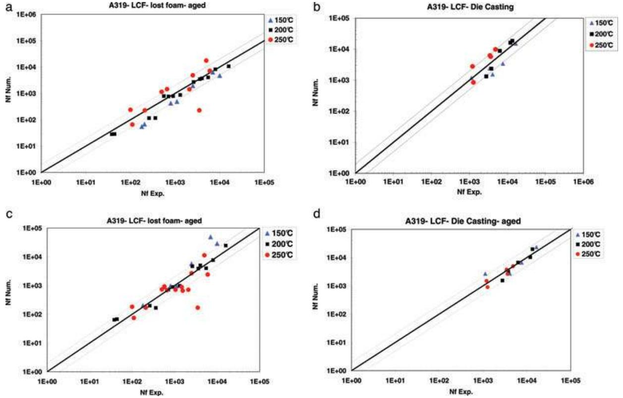
**Fig. 7** Experimental fatigue life versus predicted fatigue life: (a)  $W_{E\sigma\Delta\epsilon}$  criterion for A319-LFC, (b)  $W_{E\sigma\Delta\epsilon}$  criterion for A319-DC, (c)  $W$  criterion for A319-LFC, (d)  $W$  criterion for A319-DC.
