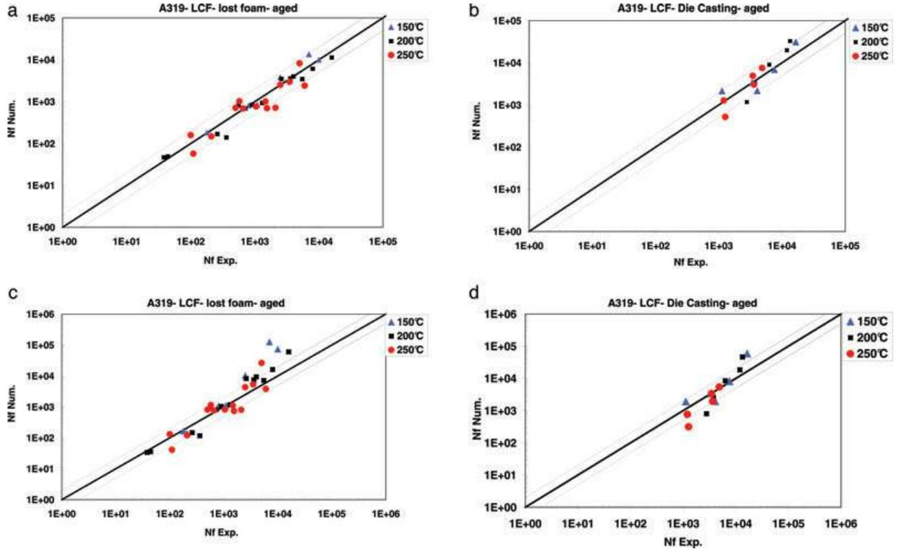
**Fig. 9** Experimental fatigue life versus predicted fatigue life: (a)  $W_{\sigma_H}$  criterion for A319-LFC, (b)  $W_{\sigma_H}$  criterion for A319-DC, (c)  $W_{\sigma_{eff}}$  criterion for A319-LFC, (d)  $W_{\sigma_{eff}}$  criterion for A319-DC.
