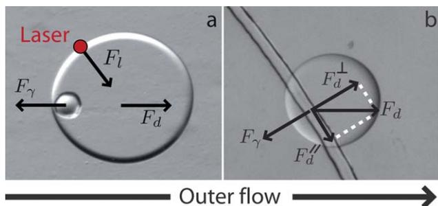
**Fig. 1** Forces acting on a drop in the presence of surface patterning: The anchoring force due to the surface patterning  $F_\gamma$ , the drag force due to the flow of the outer fluid  $F_d$ , and the force due to the laser heating  $F_l$ . (a) The case of an anchor. (b) In the case of a rail, the unbalanced force due to the drag parallel to the rail  $F_d''$  leads to motion along this direction.
