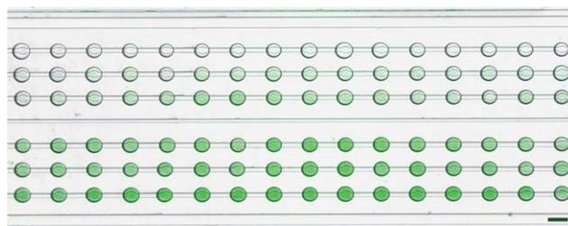
**Fig. 4** A superposition of bright-field and fluorescent images of a 96 anchor array. The droplet composition has been altered from pure water to a solution of water and green fluorescent beads to create a gradient. The droplet volume is 7 nL each. The scale bar is 300  $\mu\text{m}$ .
