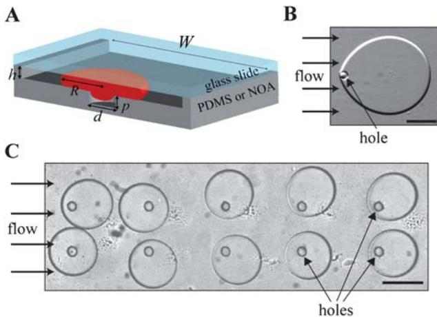
**Fig. 1** (A) Sketch of the experimental device which defines the geometric parameters. (B) A water drop anchored to a hole in the channel roof with oil flowing left to right. (C) An array of anchored droplets. The scale bar represents 250  $\mu\text{m}$  in all images.
