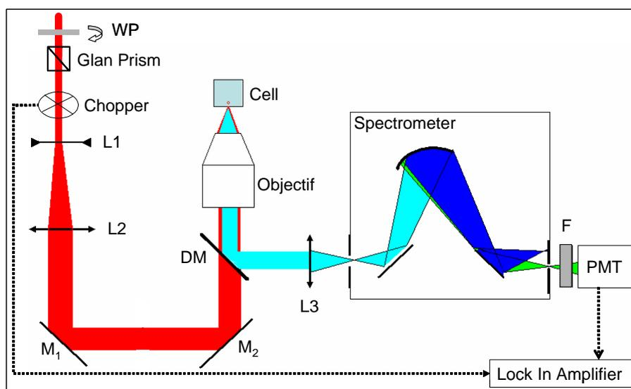
Fig. 1. 2-photon spectrofluorimeter. WP: rotating half waveplate; L1, L2, L3: lenses; M<sub>1</sub>, M<sub>2</sub>: silver mirrors; DM: dichroic mirror; F: optical filters; PMT: photomultiplier tube.
