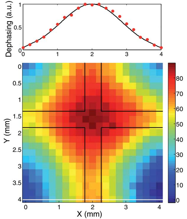
Fig. 2. (Color online) Differential spectral phase image at 1 THz of an aluminum cross ( $500 \mu\text{m}$ -large, 1 mm-deep, solid black lines).  $\alpha = 42^\circ$ . Color bar unit is degree. Top graph is a cross-section (white horizontal line) with experimental data (dots) and Gaussian convolution fit (solid).
