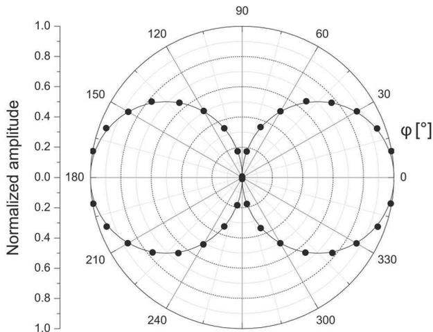
Fig. 4. Normalized amplitude of the signal from polarimetry measurements versus the angle  $\phi$  of the fixed polarizer in polar coordinates. The spectral component is at 1 THz. Filled circles, data; solid curve, theoretical fit.
