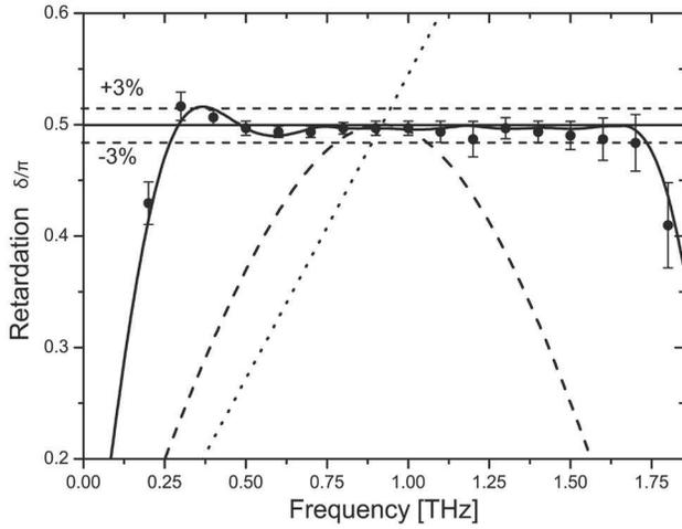
Fig. 1. Frequency dependence retardation of standard and TAQ quarter-wave plates. Relative bandwidth  $\delta\nu/\nu$  is given at 3% bandwidth (horizontal lines). Comparison with a standard birefringent wave plate (dotted curve); two-plate combination (dashed curve) and the six-plate TAQ wave plate (solid curve, calculation; filled circles, data).
