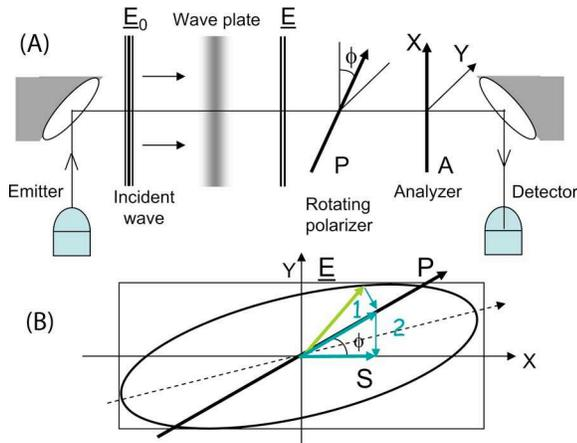
Fig. 3. (Color online) (A) Setup for polarimetry measurements of the wave plate. (B) Projection of the electric field  $E$  on the rotating polarizer and fixed analyzer gives the measured signal  $S(\phi)$ .
