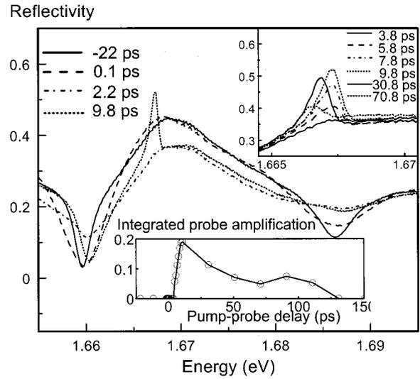
FIG. 2. Selected reflectivity spectra at  $T=80$  K for different pump-probe delays and for a pump excitation density of  $3.75 \mu\text{J}/\text{cm}^2$ . The upper inset is a blow-up of the spectral region where the probe amplification is observed. The lower inset shows the spectrally integrated probe amplification in arbitrary units as a function of pump-probe delay.
