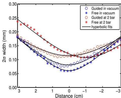
FIG. 2. (Color online) Second moment ( $2\sigma$ ) widths of the beam near the geometrical focus measured in vacuum and at 2 bar for a TM mode along the guided or free dimension, respectively, all fitted by hyperbolic curves.
