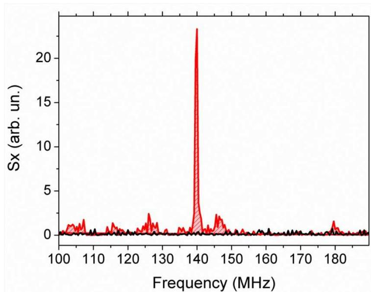
FIG. 4. Power spectral density  $S_x$  for an injected frequency  $F = 140$  MHz. Black curve is the ambient white-noise without guided discharge but with RF feeding in the solenoid coil at 140 MHz, showing perfect shielding. The guided discharge has a length  $D = 96$  cm.
