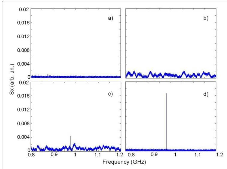
FIG. 3. Power spectral density  $S_x$  for an injected frequency  $F = 970$  MHz, for an interelectrode distance  $D = 5$  cm and a DC bias voltage  $V \approx 40$  kV. a) Signal detected with RF source on but no discharge, b) signal in the presence of discharge but without RF, c) signal with discharge and RF, d) signal obtained when the discharge is replaced by a metallic copper rod.
