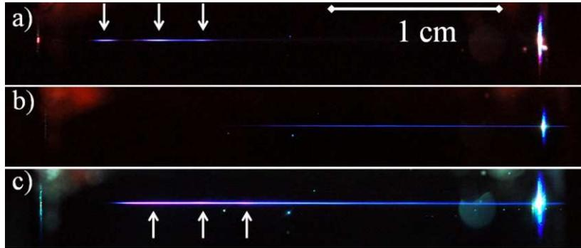
FIG. 1. Side view photography of the blue fluorescence of  $\text{SiO}_2$  induced by a self-guided laser pulse at a) 800 nm with  $P = 18 P_{cr}$ , b) 1.9  $\mu\text{m}$  with  $P = 13 P_{cr}$  and c) 1.9  $\mu\text{m}$  with  $P = 30 P_{cr}$ . The laser pulse is focused on a 70  $\mu\text{m}$  spot (FWHM) at the left surface of the 3 cm thick sample. Vertical arrows indicate the position of focusing-defocusing cycles.
