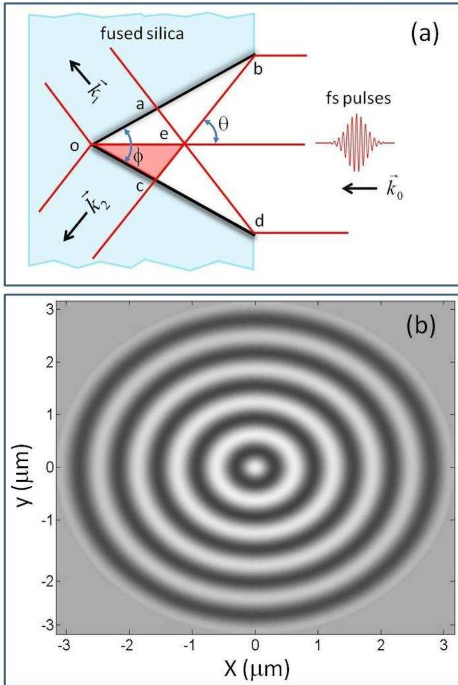
Fig. 4. (a) Schematic of the model. (b) Calculated intensity distribution of the interference laser field on the inner side surface of the damage crater.
