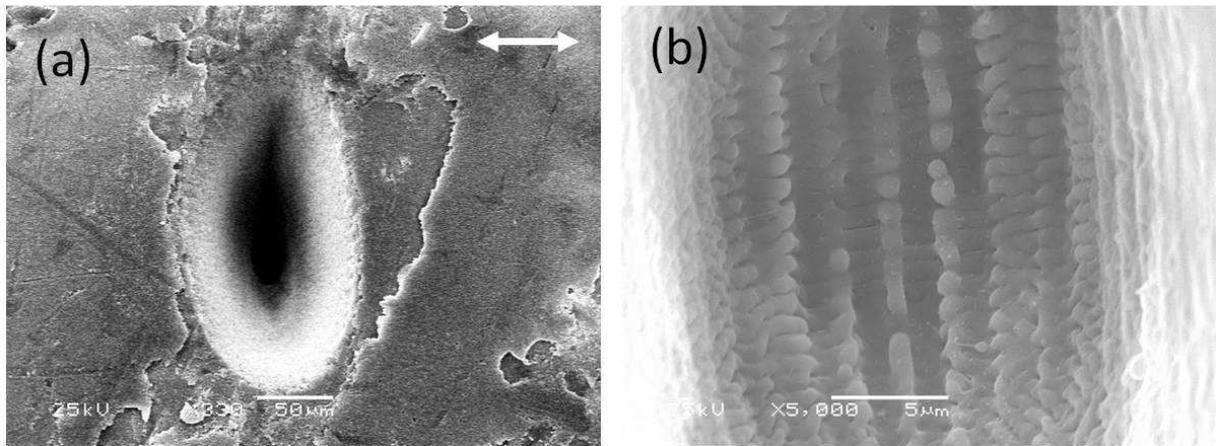
Fig. 5. The laser pulses are focused by  $f = 1000$  mm lens with additional astigmatism. (a) Whole view of the damage crater. The arrow represents the polarization direction of the laser pulse. (b) Higher resolution SEM image of the central section of (a). Vertical fringe structure with period around  $2\text{-}3\ \mu\text{m}$  is clear, in addition to the horizontal LIPSS with period of  $\Lambda \sim 0.7\ \mu\text{m}$ .
