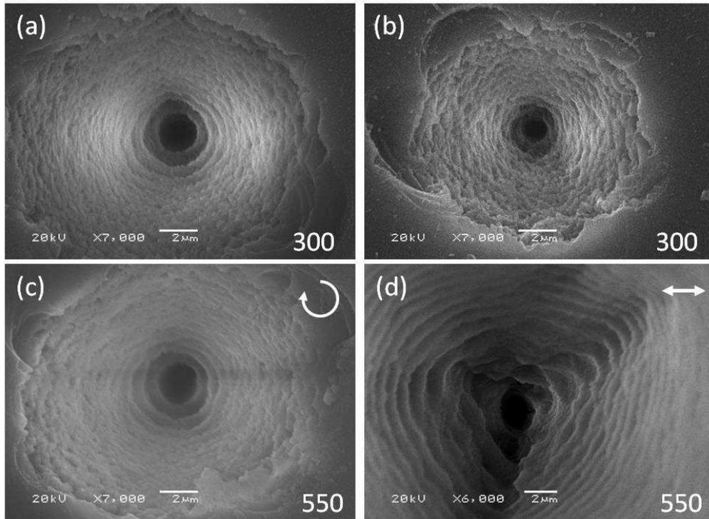
Fig. 2. The incident pulse energies are  $19\ \mu\text{J}$  and  $9\ \mu\text{J}$  for (a) and (b). The other experimental conditions are identical to those in Fig. 1. (c) The laser polarization is changed to circular. (d) The focal length is  $f=1000\ \text{mm}$  and the incident pulse energy is  $300\ \mu\text{J}$ . In each panel, the numbers indicate the laser shot number. In (c) and (d), the arrows present the polarization state of the laser pulses.
