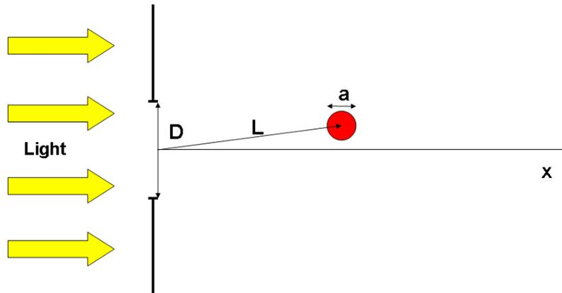
Fig. 1. Principle of near field imaging with aperture
