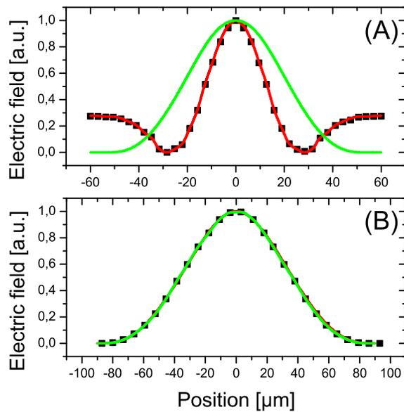
Fig. 7. Evolution of the normalized transmitted electric field versus the axon position in TNF conditions (A,  $L=80\mu\text{m}$ ) and with CNF conditions (B,  $L=140\mu\text{m}$ ). The black dots are the experimental data, the red line is the full 3D FEM simulation fit, and the green line is the GFP fit.
