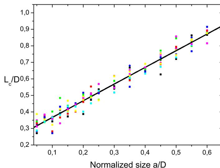
Fig. 3. Evolution of the normalized distance  $L_c/D$  versus  $a/D$ . The point color is related to  $D/\lambda$ : black for  $1/3$ , red for  $1/4$ , green for  $1/5$ , blue for  $1/6$ , cyan for  $1/7$ , magenta for  $1/8$ , yellow for  $1/9$ . The black line is the linear fit of the simulations. The shape of points is related to the simulation, circles for  $\nabla_M$  and squares for  $\Delta$
