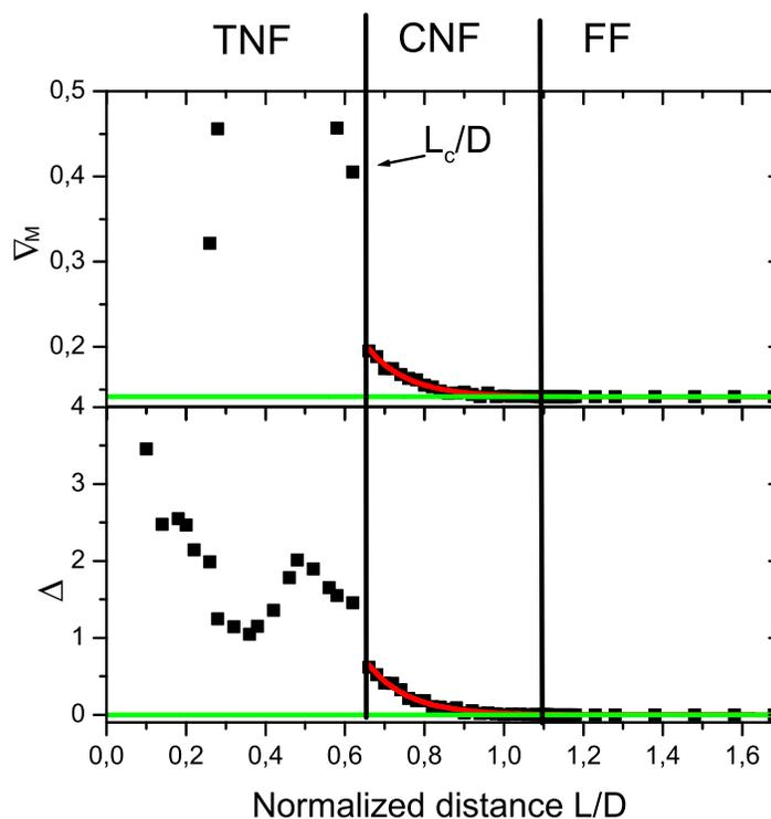
Fig. 2. Example for a spherical sample of normalized size 0.2 of the evolution of  $\nabla_M$  and  $\Delta$  with normalized distance  $L/D$ . Three domains have been pointed out: the true near field domain (TNF), the contrast near field domain (CNF), and the far field domain (FF). The red lines are the exponential fits in the CNF domain. The green lines are FF references.
