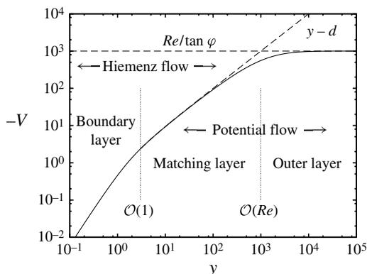
FIGURE 2. Wall-normal component  $V(y)$  of the uniformly valid base-flow solution around a swept cylinder for  $Re = 1000$  and  $\varphi = 45^\circ$ . The stagnation-point flow in the matching layer and the oncoming parallel flow in the outer layer are indicated with dashed lines.
