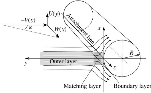
FIGURE 1. Flow around a swept cylinder with radius  $R$  and sweep angle  $\varphi$ . The  $x$ -axis is oriented in the chordwise direction, the wall-normal  $y$ -axis points in the upstream direction, and the spanwise  $z$ -axis coincides with the attachment line.
