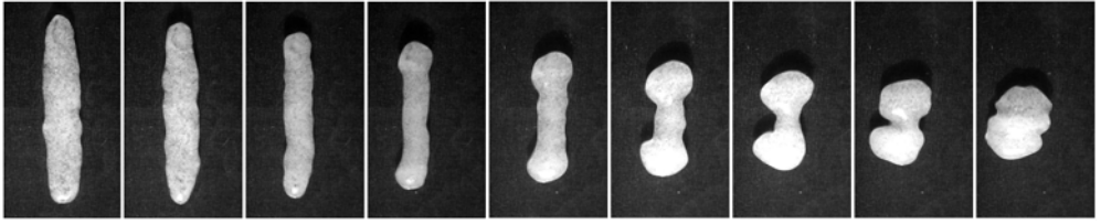
FIGURE 7. Top view of the retraction of a liquid ribbon of initial length 22.5 mm, width 4 mm and height 2.2 mm. The ribbon retracts from its two ends, without developing a Plateau–Rayleigh instability. Time interval between images: 12 ms.
