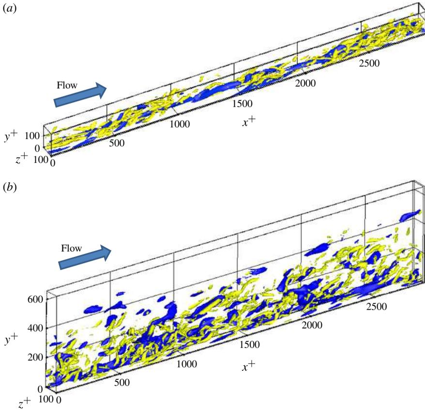
FIGURE 7. (Colour online) Instantaneous streamwise velocity fluctuations (dark grey/blue online) and vortical structures (light grey/yellow online) of (a)  $N180$  ( $u^+ = -2.5$ ,  $\mathbf{Q}^+ = 0.0089$ ) and (b)  $N660$  ( $u^+ = -2.5$ ,  $\mathbf{Q}^+ = 0.016$ ).
