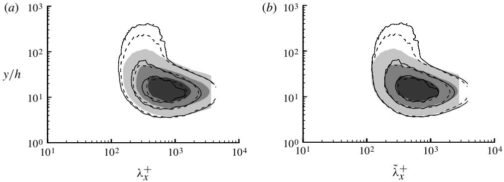
FIGURE 9. Premultiplied streamwise spectra of the streamwise velocity (a) before and (b) after the correction (A 1): shaded,  $N180$ ; dashed,  $N410$ ; solid,  $N660$ . The contour labels are chosen as 0.25, 0.5 and 0.75 times the maximum.
