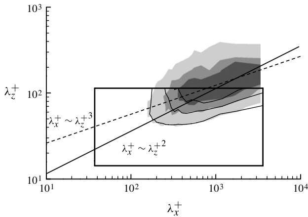
FIGURE 10. Two-dimensional spectra of the streamwise velocity, where the shaded and solid contours are, respectively, from  $F180$  and  $N180$ . Here, the solid and dashed lines indicate  $\lambda_x^+ \sim \lambda_z^{+2}$  and  $\lambda_x^+ \sim \lambda_z^{+3}$ , respectively.
