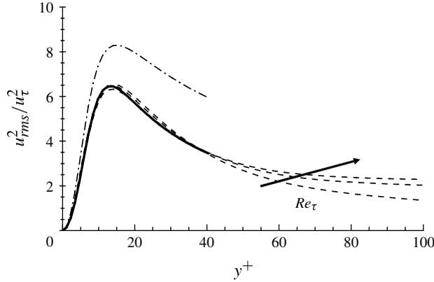
FIGURE 8. Streamwise turbulent kinetic energy profiles: ----, the filtered simulations ( $N180$ ,  $N410$  and  $N660$ ); —,  $f_1(y^+)$  with the fitting constants in (4.2); - · - · -,  $f_1(y^+)$  with the fitting constants in Marusic & Kunkel (2003).
