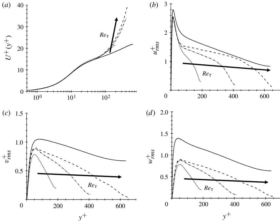
FIGURE 3. (a) Mean velocity profile  $U^+(y^+)$  and turbulent velocity fluctuations (b)  $u_{rms}^+(y^+)$ , (c)  $v_{rms}^+(y^+)$  and (d)  $w_{rms}^+(y^+)$ . Curves: —, DNS by Abe *et al.* (2004) at  $Re_\tau = 640$ ;  $\cdots\cdots$ ,  $N180$ ;  $-\cdot-\cdot-$ ,  $N410$ ;  $-----$ ,  $N660$ .
