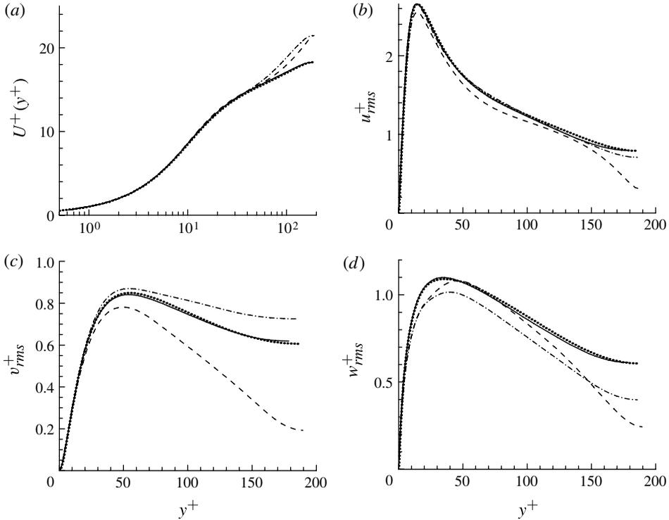
FIGURE 1. (a) Mean velocity profile  $U^+(y^+)$  and turbulent velocity fluctuations (b)  $u_{rms}^+(y^+)$ , (c)  $v_{rms}^+(y^+)$  and (d)  $w_{rms}^+(y^+)$ . Curves: —, *F180*; ·····, DNS by del Álamo *et al.* (2004); - · - · -, *S180* (spanwise minimal domain only); ---, *N180* (spanwise minimal domain with the filtering (2.2)).
