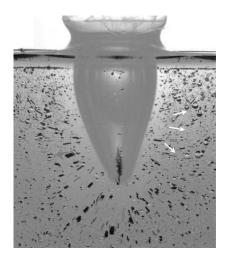
FIG. 5. Visualisation of the flow around the cavity created by a polypropylene sphere with  $R_0 = 2.5$  mm and  $V_0 = 24$  m/s. The motion in the oil is visualized using small trapped air bubbles and superimposing 1.6 ms of experiment. The white arrows underline the direction of the velocity vector. The image is taken 3 ms after impact.
