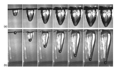
FIG. 7. Chronophotography of the impact of two spheres with  $R_0 = 2.5$  mm,  $V_0 = 13$  m/s, and different densities: (a) polypropylene,  $\rho_s = 920$  kg/m<sup>3</sup> and (b) stainless steel,  $\rho_s = 7700$  kg/m<sup>3</sup>.
