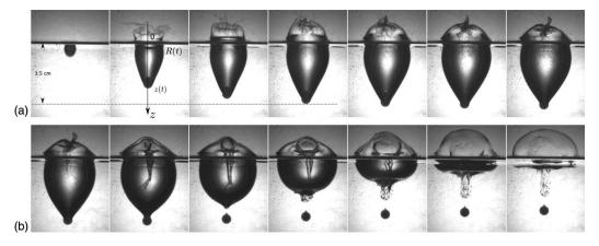
FIG. 2. Chronophotography of the impact of a polypropylene sphere (radius  $R_0 = 3.5$  mm) onto a bath of silicon oil ( $\eta = 1000$  mPa s) at  $V_0 = 28$  m/s. The first row of pictures shows the rapid opening of the cavity (interval  $\Delta t$  between two snapshots is 2.8 ms), while the second row represents its slower decay ( $\Delta t = 16$  ms) (movie is slowed down 250 times) (enhanced online). [URL: http://dx.doi.org/10.1063/1.4797499.1]
