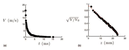
FIG. 3. Deceleration of a polypropylene sphere ( $R_0 = 2.5$  mm) arriving at  $V_0 = 20$  m/s onto a bath of silicon oil ( $\eta = 1$  Pa s): the velocity is plotted as a function of time t in (a) and the quantity  $\sqrt{V/V_0}$  as a function of distance z in (b). The dashed line represents the best linear fit (Eq. (2)), with  $z^* \approx 26$  mm.
