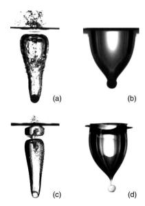
FIG. 1. (a) and (b) Cavities created by a polypropylene sphere of radius  $R_0 = 2.4$  mm impacting at  $V_0 = 15$  m/s a bath of silicon oil of viscosity (a)  $\eta = 10$  mPa s and (b)  $\eta = 1000$  mPa s. (c) and (d) Cavities created by a glass sphere of radius  $R_0 = 2$  mm after an impact at  $V_0 = 18$  m/s onto a bath (c) of water ( $\eta = 1$  mPa s) or (d) of pure glycerol ( $\eta = 1400$  mPa s).
