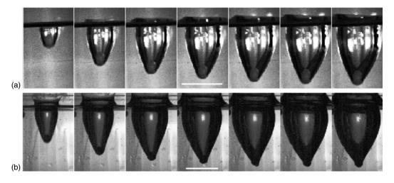
FIG. 6. Chronophotographies of the cavity after the impact of a polypropylene sphere ( $R_0 = 2.5 \text{ mm}$ ,  $\rho_s = 920 \text{ kg/m}^3$ ) at different velocities: (a)  $V_0 = 12.8 \text{ m/s}$  with  $\Delta t = 1.4 \text{ ms}$  and (b)  $V_0 = 25.9 \text{ m/s}$  with  $\Delta t = 1.25 \text{ ms}$ . The bars indicate 2 cm.
