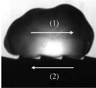
FIG. 6. Linke's device: A Leidenfrost drop made of water or ethanol on a hot surface with asymmetric teeth self-propels in direction (1). The teeth are 1.5 mm wide and 200  $\mu\text{m}$  high, and the surface temperature is 350  $^{\circ}\text{C}$ . After accelerating for a few centimeters, the drop reaches a constant velocity  $V = 14$  cm/s, fixed by the friction in direction (2) [7].
