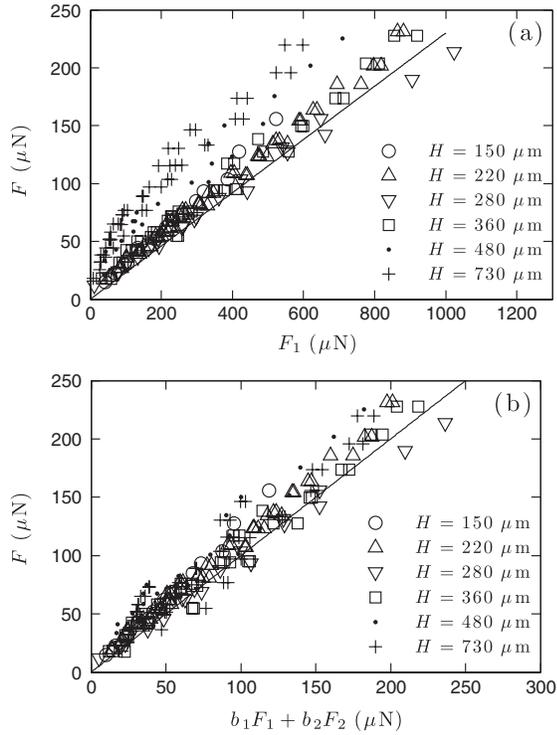
FIG. 5. (a) Measured friction force  $F$  as a function of  $F_1 = \rho R^2 V^2 \frac{H}{\lambda}$ ; the straight line has a slope of  $b_1 = 1.4$ . (b) Friction force  $F$  as a function of  $b_1 F_1 + b_2 F_2$  with  $b_1 = 1.4$  [deduced from (a)],  $F_2 = \rho g R^2 \frac{H^2}{\lambda^2}$ , and  $b_2 = 2.9$ . The straight line has a slope of 1.
