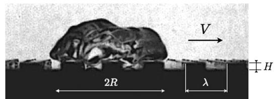
FIG. 1. Ethanol drop ( $\Omega = 150\ \mu\text{L}$ ) sliding on aluminum crenelations of wavelength  $\lambda = 3\ \text{mm}$  and height  $H = 480\ \mu\text{m}$ . The solid is at a temperature of  $450\ ^\circ\text{C}$ , and the drop moves at a velocity  $V = 19\ \text{cm/s}$ .
