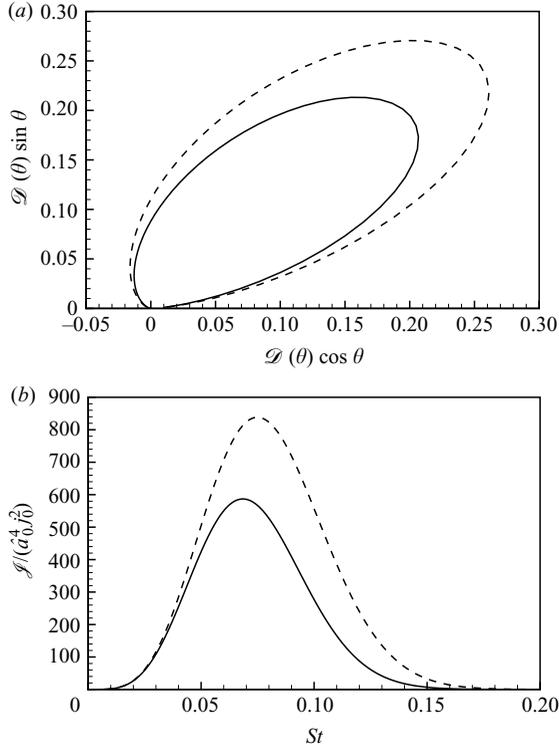
FIGURE 7. (a) The directivity and (b) the spectrum at  $\theta = 90^\circ$  of the acoustic field radiated by a linear wavepacket with  $St = 0.44$  and  $\Delta\omega = 0.5$ . Solid lines: non-equilibrium result; dashed lines: equilibrium result. Reynolds number  $R = 1800$  and  $\sigma_s = 0.043$ .
