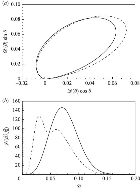
FIGURE 9. Effect of the Reynolds number on the (a) directivity and (b) spectrum of the acoustic field radiated by a linear wavepacket with  $St = 0.44$ ,  $\Delta\omega = 0.3$  and  $\sigma_s = 0.043$ . Solid lines:  $R = 1800$ ; dashed lines:  $R = 2.7 \times 10^5$ .
