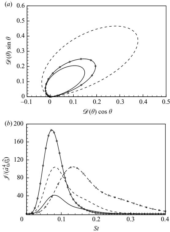
FIGURE 11. The (a) directivity and (b) spectrum of a linear wavepacket with  $St = 1.0$  at Reynolds number  $R = 2.7 \times 10^5$ . Solid lines:  $\sigma_s = 0.043$  and  $\Delta\omega = 0.5$ ; solid lines with symbols:  $\sigma_s = 0.0215$  and  $\Delta\omega = 0.5$ ; dashed lines without symbols:  $\sigma_s = 0.043$  and  $\Delta\omega = 0.8$ . In (b), the dashed line with symbols represents the spectrum at  $\theta_p = 53^\circ$  ( $\sigma_s = 0.043$  and  $\Delta\omega = 0.8$ ).
