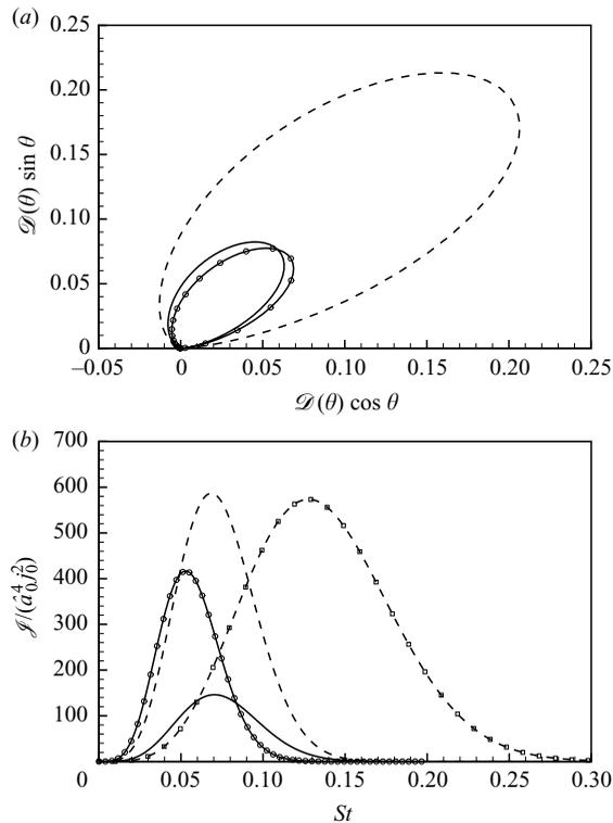
FIGURE 8. The (a) directivity and (b) spectrum of the acoustic field radiated by a linear wavepacket with  $St=0.44$  at  $R=1800$ . Solid lines:  $\sigma_s=0.043$  and  $\Delta\omega=0.3$ ; solid lines with symbols:  $\sigma_s=0.0215$  and  $\Delta\omega=0.3$ ; dashed lines without symbols:  $\sigma_s=0.043$  and  $\Delta\omega=0.5$ . In (b), the dashed line with symbols represents the spectrum at  $\theta=46^\circ$  ( $\sigma_s=0.043$  and  $\Delta\omega=0.5$ ).
