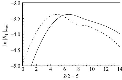
FIGURE 5. The axial distribution of the peak density fluctuation  $R_1 \equiv \epsilon R^{-1/3}(-\Theta_1/T_c^2)$  (solid line) of a mode with  $St = 0.44$  and  $a_0 = 7.61 \times 10^{-3}$  and comparison with the amplitude development (dashed line). The axial coordinate is the distance to the jet exit normalized by the diameter.
