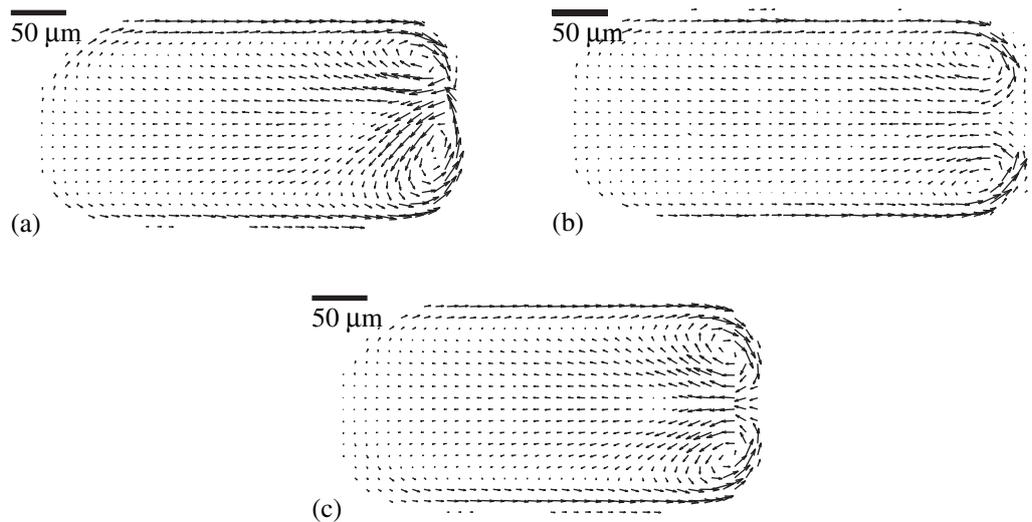
**Figure 4.** Velocity fields obtained with (a) one off-center laser beam, (b) two rapidly alternating laser spots and (c) the superimposition of the first velocity field and its mirror image with respect to the center plane of the drop.
