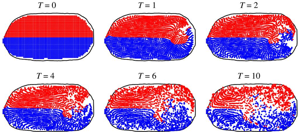
**Figure 9.** Snapshots of the position of passive tracers as a function of time. Blue (red) spots represent particles placed in the lower (upper) part of the drop at  $t = 0$ ,  $D = 102 \mu\text{m}$  and  $\tau_{\text{laser}} = 100 \text{ ms}$ .
