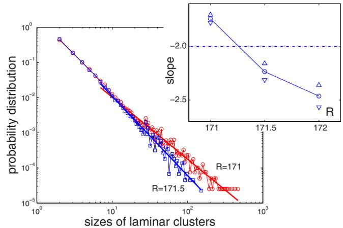
FIG. 3. (Color online) Main: Probability distribution of cluster areas (numbers of laminar pixels). Inset: Variation of the slope of the distribution tails with  $R$ ; up and down arrow heads indicate error bar on the slope.
