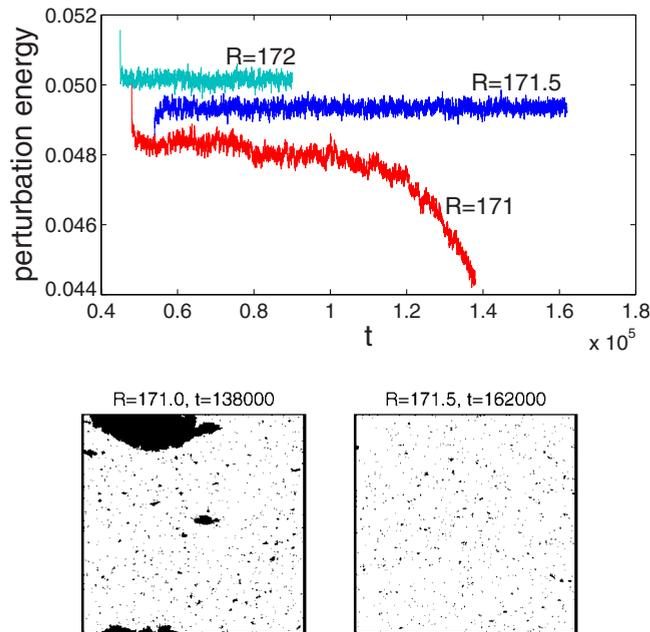
FIG. 2. (Color online) Top: time series of  $E_t$  for the extrawide domain  $\mathcal{D}=1536 \times 1536$ . Bottom: two black and white snapshots of the solution for  $R=171$  (left) and 171.5 (right). Thresholding performed according to the rule given in the text.
