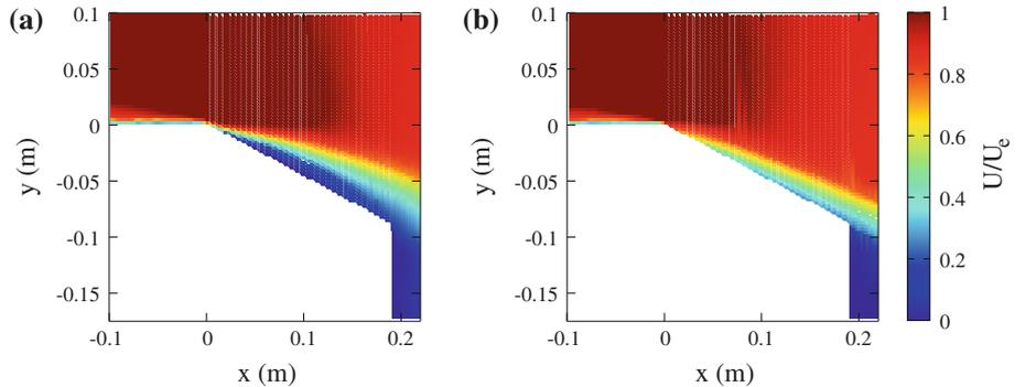
bubble. When control is applied, the shear layer becomes thinner and its curvature is highly reduced. This behavior suggests that the re-circulation bubble has been suppressed or at least highly reduced.
