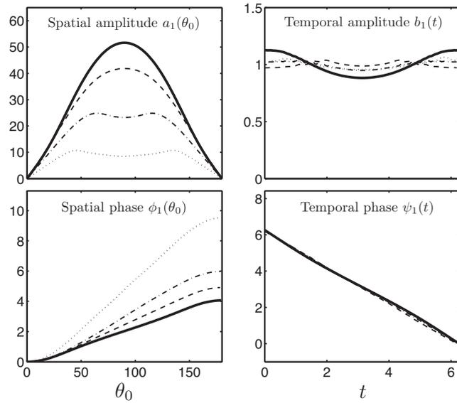
FIG. 18. Amplitude and phase characteristics of the dominant CEOF mode in the unconstrained swimming stroke of maximum efficiency (thick solid line:  $\Theta_{\max} \approx 52.6^\circ$  and  $\eta \approx 22.2\%$ ) and in constrained optimal strokes (thin lines):  $\Theta_{\max} \approx 44^\circ$  and  $\eta \approx 21\%$  (dashed),  $\Theta_{\max} \approx 25^\circ$  and  $\eta \approx 12.5\%$  (dashed-dotted),  $\Theta_{\max} \approx 11^\circ$  and  $\eta \approx 6.8\%$  (dotted).
