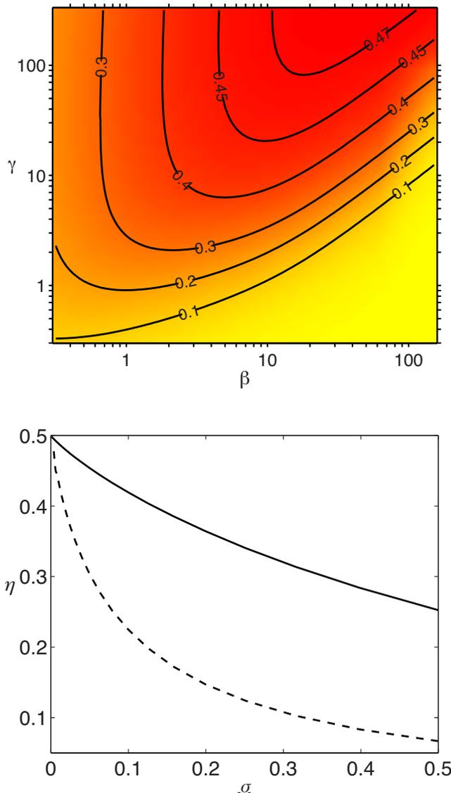
FIG. 13. (Color online) (Top) Variations of the swimming efficiency obtained for the analytical *ansatz*, for a sweep in the  $(\beta, \gamma)$  parameter space, and a shock width parameter of  $\sigma=0.05$ ; lines display isovalues of  $\eta$ . (Bottom) Evolution with  $\sigma$  of the efficiency of the analytical *ansatz* for  $\gamma=1000$  (solid) and  $\gamma=200$  (dashed); in both cases  $\beta=800$ .
