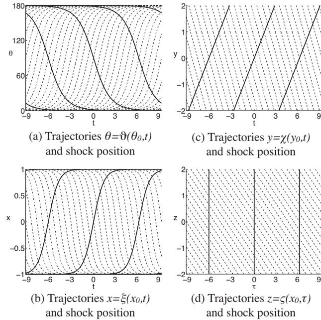
FIG. 12. The construction of the analytical *ansatz* is illustrated in the four successive coordinate systems used (a)  $(t, \theta)$ , (b)  $(t, x)$ , (c)  $(t, y)$ , and (d)  $(\tau, z)$ . The trajectories corresponding to the outer solution are shown in dashed lines and thick solid lines show the position of the shocks and inner solution trajectories [Eq. (55)]. Here,  $\gamma=1$  and  $\beta=0.7$ , and three swimming periods are shown.
