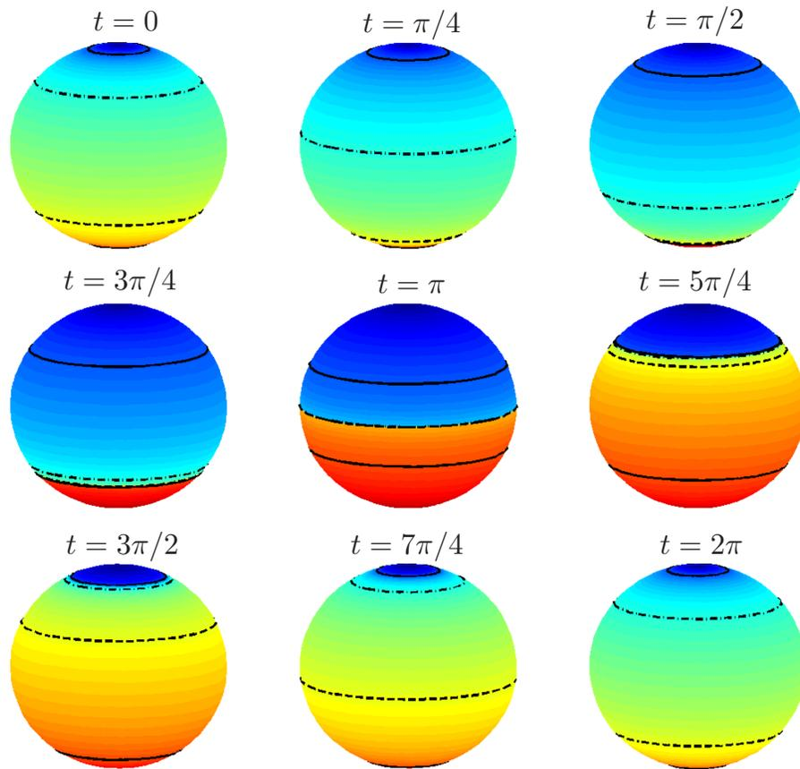
FIG. 5. (Color online) Snapshots of the displacement of the squirmer surface over a swimming period in the optimal unconstrained stroke ( $\Theta_{\max} \approx 52.6^\circ$ ,  $\langle U \rangle \approx 0.33$ ,  $\eta \approx 22.2\%$ ). The surface color of each material point on the surface refers to the mean polar angle of that material point. Black lines also correspond to the location of particular material points and have been added for clarity.
