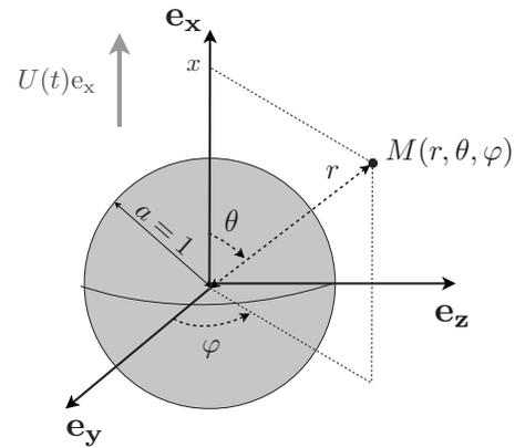
FIG. 2. Notation for the squirmer model. A comoving frame centered on the squirmer center is used with spherical polar coordinates  $(r, \theta, \varphi)$ . The axisymmetry of the surface motion imposes a purely translating swimming motion along  $\mathbf{e}_x$  with time-varying velocity  $U(t)$ . See text for details.
