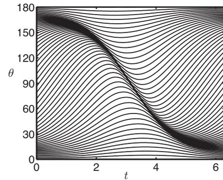
FIG. 4. Lagrangian description of the optimal swimming stroke with no constraint on the maximum displacement. The maximum amplitude of displacement is  $\Theta_{\max} \approx 52.6^\circ$ , the mean swimming velocity is  $\langle U \rangle \approx 0.33$ , and the swimming efficiency is  $\eta \approx 22.2\%$ . Each curve illustrates the trajectory  $\theta = \vartheta(\theta_0, t)$  of a single material surface point.
