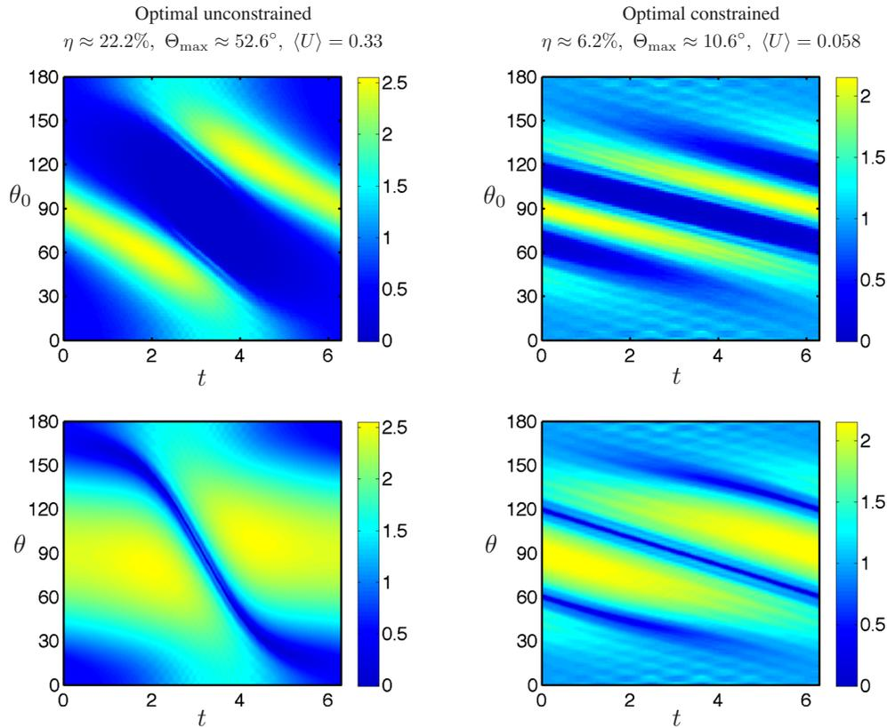
FIG. 15. (Color online) (Top) Lagrangian map in the  $(\theta_0, t)$  plane and (bottom) Eulerian map in the  $(\theta, t)$  plane of the stretching parameter  $S$  for the unconstrained swimming stroke (left) and the result of constrained optimization with efficiency 6.2% and maximum displacement  $10.6^\circ$  (right).
