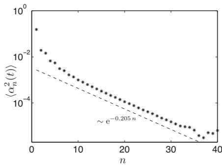
FIG. 3. The contribution of the successive modes,  $\langle \alpha_n^2 \rangle$ , to the efficiency (stars) decreases exponentially with the mode order,  $n$ . The results are plotted for the unconstrained optimization with efficiency  $\eta \approx 22.2\%$  and were obtained with  $M=40$ ,  $N_x=150$ , and  $N_t=128$ .
