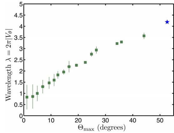
FIG. 19. (Color online) Variation of the wavelength  $\lambda$  (or phase velocity  $|V_\theta| = \lambda/2\pi$ ) measured along the surface of the spherical swimmer, with the maximum angular displacement,  $\Theta_{\max}$ . The star (blue online) corresponds to the unconstrained optimal swimming stroke of Sec. II.
