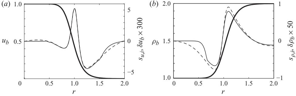
FIGURE 2. Baseflow profiles (3.1) and (3.2) with parameters  $b_u = b_\rho = 0.1$ ,  $d = 0$ ,  $S = 0.5$ , constrained optimal variations and sensitivities of the absolute growth rate. (a) —, velocity  $u_b$ ; —, variation  $\delta u_b$ ; - -, sensitivity  $s_{u,i} = \text{Im}(s_u)$ ; (b) —, density  $\rho_b$ ; —, variation  $\delta \rho_b$ ; - -, sensitivity  $s_{\rho,i} = \text{Im}(s_\rho)$ .
