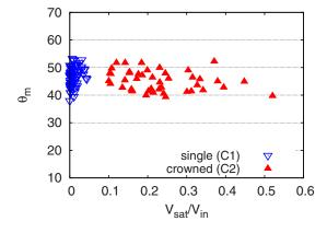
FIG. 7. (Color online) Measured opening angles  $\theta_m$  of single and crowned cap bubbles plotted vs the ratio  $V_{\rm sat}/V_{\rm in}$ . The data used to generate this figure are available online as supplemental material (Ref. 14).
