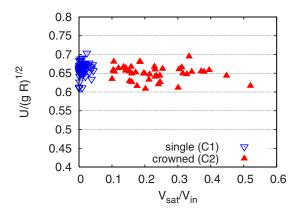
FIG. 6. (Color online) Measured individual Davies and Taylor ratios  $U/\sqrt{gR}$  of single and crowned cap bubbles plotted vs the ratio of the estimated volume  $V_{\rm sat}$  contained in the satellite bubbles to the total injected volume of gas  $V_{\rm in}$ . The ratio predicted by the theory of Davies and Taylor (Ref. 11) is  $2/3 = 0.666\bar{6}$ . The data used to generate this figure are available online as supplemental material (Ref. 14).
