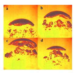
FIG. 3. (Color online) Pictures of typical crowned cap bubbles with, respectively, (a)  $V_{\rm in}$ =114 cm³,  $V_{\rm sat}/V_{\rm in}$ =0.05; (b)  $V_{\rm in}$ =126 cm³,  $V_{\rm sat}/V_{\rm in}$ =0.15; (c)  $V_{\rm in}$ =144 cm³,  $V_{\rm sat}/V_{\rm in}$ =0.3; and (d)  $V_{\rm in}$ =66 cm³,  $V_{\rm sat}/V_{\rm in}$ =0.5.
