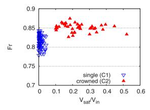
FIG. 5. (Color online) Measured individual Froude numbers of single and crowned cap bubbles plotted vs the ratio of the estimated volume  $V_{\rm sat}$  contained in the satellite bubbles to the total injected volume of gas  $V_{\rm in}$ . The data used to generate this figure are available online as supplemental material (Ref. 14).
