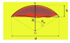
FIG. 2. (Color online) Geometry of a single spherical cap bubble. Picture of a single spherical cap bubble of air  $(V=68~{\rm cm^3})$  rising in still water at constant speed U. R is the radius of curvature of the bubble at the front stagnation point S, while  $\theta_m$  is its subtended half-angle; h and d are the height and width of the bubble, respectively.
