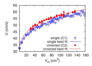
FIG. 4. (Color online) Rise speed U vs total injected volume of air for single cap bubbles ( $V_{\rm sat}/V_{\rm in} < 0.05$ ) generated with the C1 cup and crowned cap bubbles ( $V_{\rm sat}/V_{\rm in} > 0.1$ ) generated with the C2 cup. The best-fit curves have been computed by assuming  $U={\rm Fr}\,g^{1/2}V_{\rm in}^{1/6}$  and then computing the best-fit Froude number Fr. The data used to generate this figure are available online as supplemental material (Ref. 14).
