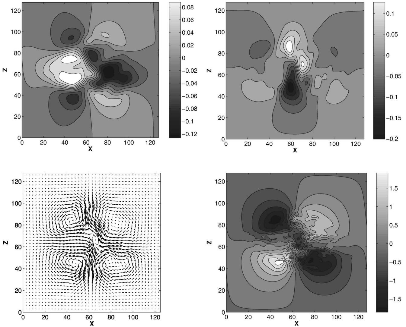
FIG. 3. Top: level lines of averaged velocity components  $\bar{U}_0$  (left) and  $\bar{W}_0$  (right), illustrating large-scale streamwise inflow and spanwise outflow around the spot. Bottom, left: representation of this flow as vectors. Bottom, right: level lines of the unfiltered stream function  $\Psi_0$ .
