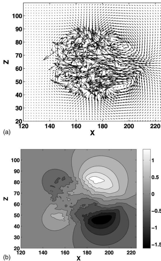
FIG. 9. (a) The flow field  $(U_0, W_0)$  exhibits a quadrupolar structure (not all the points are represented). (b) Spatial distribution of the stream function  $\Psi_0$ . Outside the spot, it has four lobes with alternating sign. Each lobe corresponds to a region of large recirculation.
