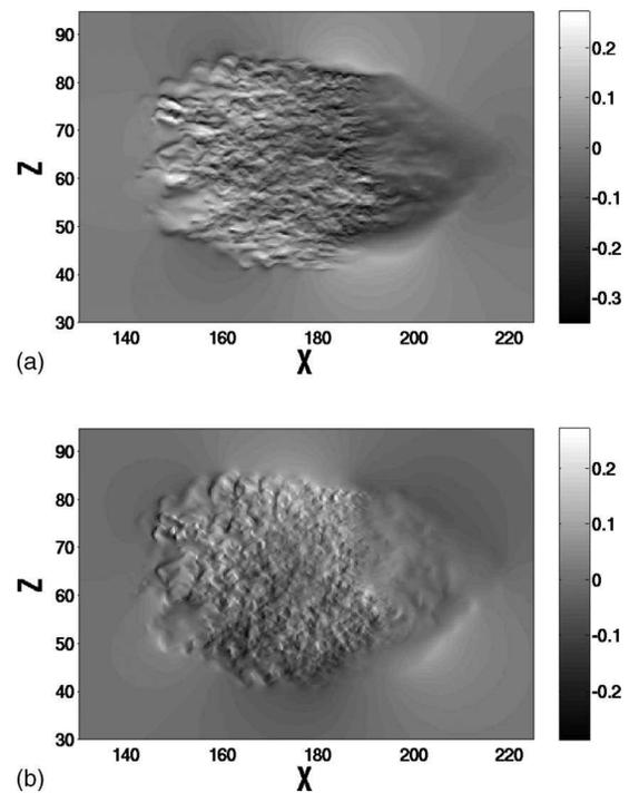
FIG. 8. The spatial distribution of  $U_0$  (a) represents an inflow toward the spot, whereas  $W_0$  (b) represents an outflow from the spot. Outside the spot, the in-plane flow  $(U_0, W_0)$  is quadrupolar, as shown in Fig. 9.
