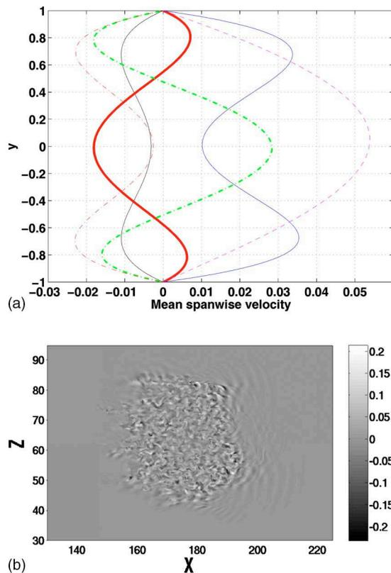
FIG. 5. (Color online) (a) The mean value of the total spanwise velocity in each upper box ( $z \geq 64$ ), shown in Fig. 4. Same color convention as in Fig. 4(b). (b) The spatial distribution of  $V_2$ . At the channel centerline, the total wall-normal velocity is equal to  $BV_2$ . Oblique waves are present at the wing tips of the spot (enhanced online).
