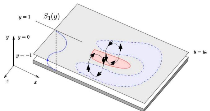
FIG. 11. (Color online) 3D reconstruction of the crescent vortex, depicted by  $V_1$  and  $(U_1, W_1)$  in Fig. 10. The distribution of  $V_1$  has a crescent shape in the shaded plane for some  $y = y_c \in [0, -1]$ . The two circles represent the cross section  $(z, y)$  of the streamwise vortices. The polynomial  $S_1$  is plotted by a solid blue line. For clarity, only the two counter-rotating streamwise vortices spanning the half-space  $y \in [-1, 0]$  are represented.
