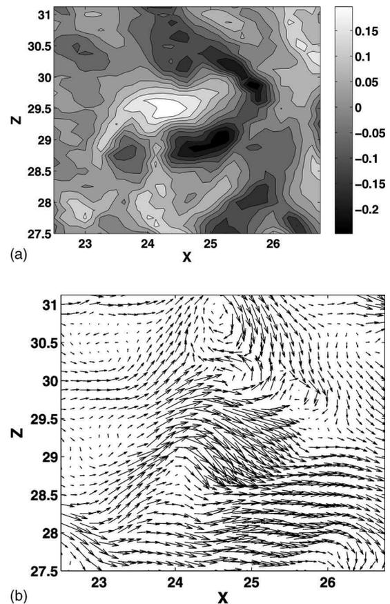
FIG. 10. Spatial distribution of  $V_1$  (a) and the flow field  $(U_1, W_1)$  (b). This spatial distribution represents a crescent vortex in each half-space  $y \in [-1, 0]$  and  $y \in [0, 1]$ . A 3D representation is given in Fig. 11. The two legs of the crescent vortex are elongated in the streamwise direction and form the streamwise vortices.
