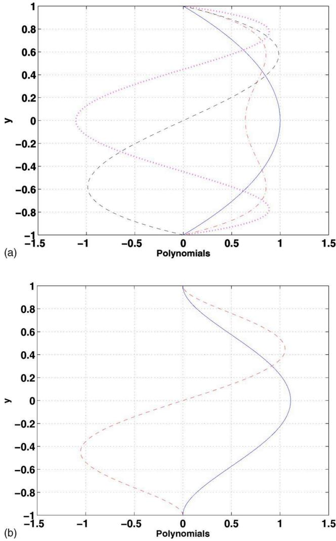
FIG. 1. (Color online) Profiles of the basis functions used in the derivation of the model. (a) Polynomials for the in-plane velocity.  $R_0$  with dash-dotted (red) line,  $R_1$  in dotted (magenta),  $R_2$  in dashed (black), and the base flow  $U(y) = U_b(1 - y^2)$  in solid (blue). (b) Polynomials for the wall-normal velocity.  $S_1$  in dashed (red) and  $S_2$  in solid (blue).
