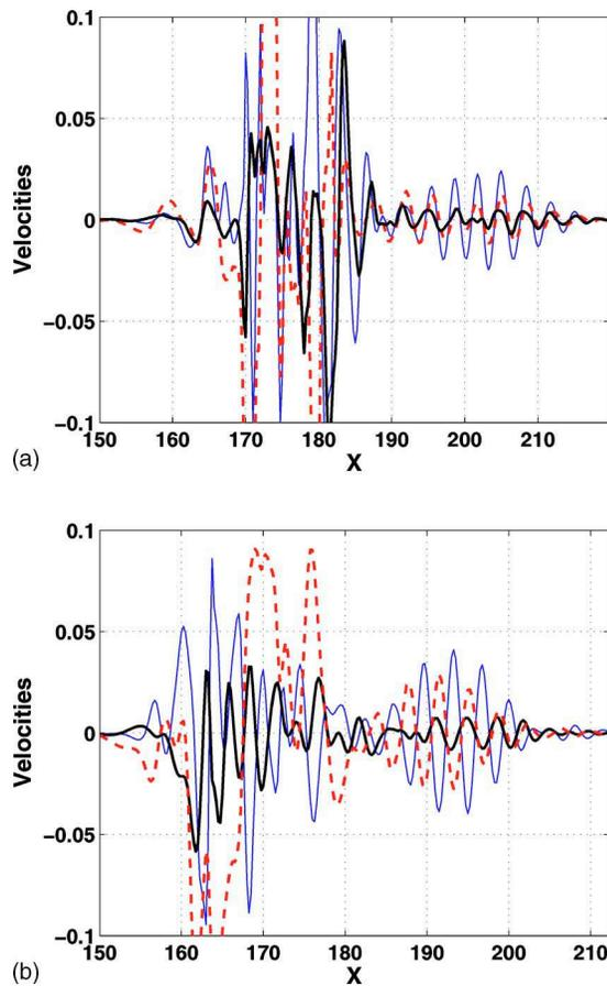
FIG. 7. (Color online) The profiles of  $U_2$  (in dashed red),  $W_2$  (in thin blue),  $V_2$  (in thick black) along a streamwise line for  $z=44$  (a) and  $z=86$  (b). The wave packets are clearly observed for  $x \in [190, 215]$  (a) and  $x \in [180, 210]$  (b).
