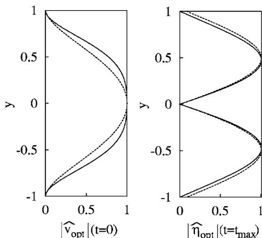
FIG. 5. Optimal initial condition  $\hat{v}_{\text{opt}}(t=0)$  and optimal response  $\hat{\eta}_{\text{opt}}(t=t_{\text{max}})$  leading to largest transient energy growth at  $\text{Re}=1500$  and for  $(\alpha, \beta)=(0, 2)$ , for both no-slip (solid line) and symmetric slip (dashed line) cases with  $\text{Kn}=0.03$ .
