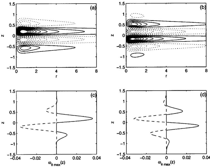
FIG. 2. Contour and extreme-value plots of  $\omega_\theta$  at  $t=0$  for  $\alpha=0.4$ ,  $F_v=0.75$ ,  $Re=100$ , (a), (c)  $Sc=700$ , and (b), (d)  $Sc=0.7$ . The dotted contours represent negative values of the solid contours positive values. The positive contour intervals and increments in (a) and (b) are  $(\omega_{\theta min} : \Delta\omega_\theta : \omega_{\theta max}) = (0.002 : 0.003 : 0.029)$ .
