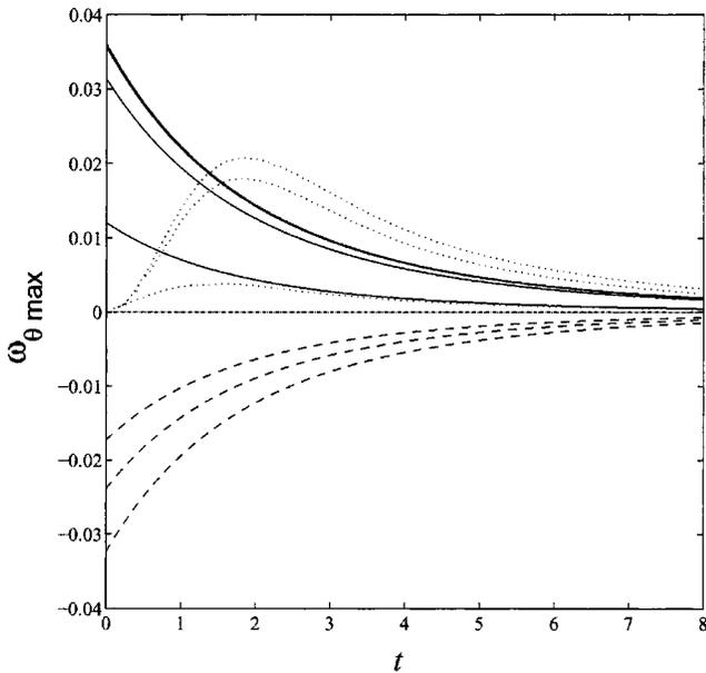
FIG. 4. Plots of  $\omega_{\theta \max}(t)$  for  $\alpha=0.4, F_v=0.75, \text{Re}=100$ . Asymptotic model results are shown in dashed and solid lines for (from bottom to top curve)  $Sc=0.7, 0.8, 0.9, 1, 10, 100$ , and  $700$ . In dotted curves the results of the BVCH numerical simulations (see the text) for  $Sc=1, 10$ , and  $100$  (from bottom to top curve).
