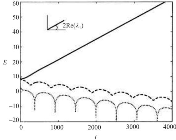
FIGURE 8. Perturbation energy  $E$  as a function of time  $t$  on a semi-log plot for  $\Omega = \Omega_B + 1$ ,  $N = 12$ ,  $\ell = 1$ . Solid line: no control, dashed line: with control; dotted line: control energy.
