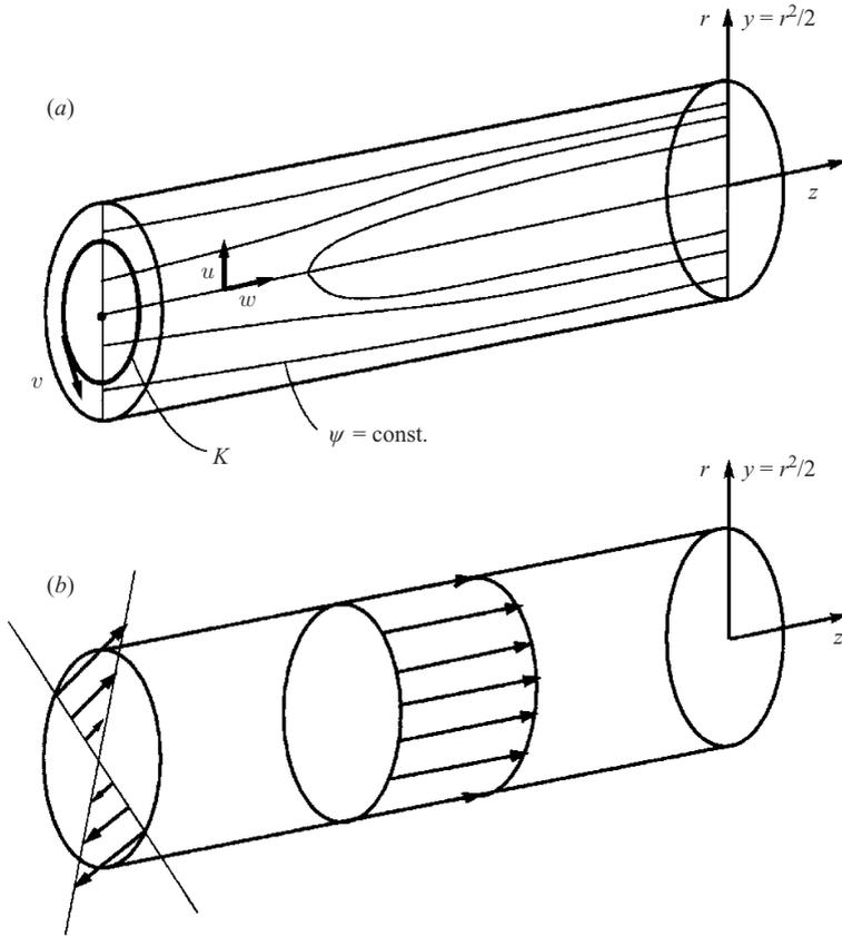
FIGURE 1. Flow configuration. (a) Sketch of breakdown state and essential flow variables; axisymmetric streamsurfaces  $\psi(y, z, t) = \text{const.}$  have been represented by their intersections with a meridional plane. (b) Base flow consisting of plug axial flow and solid body rotation.
