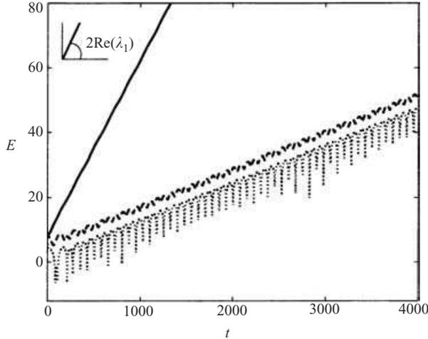
FIGURE 9. Perturbation energy  $E$  as a function of time  $t$  on a semi-log plot for  $\Omega = \Omega_B + 4$ ,  $N = 12$ ,  $\ell = 1$ . Solid line: no control, dashed line: with control; dotted line: control energy.
