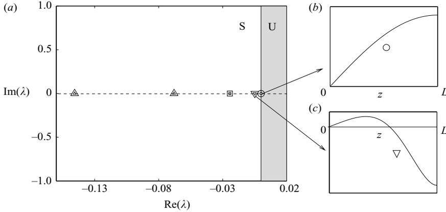
FIGURE 3. Global eigenvalue spectrum and associated eigenmodes at the swirl parameter  $\Omega = \Omega_B + 0.028$ . (a) Eigenvalues  $\lambda_i$  in complex  $\lambda$ -plane; large symbols: zeros of  $D(\lambda)$  given in (3.6); small symbols: corresponding eigenvalues of the discretized equations (5.1); note the presence of only one unstable eigenvalue  $\lambda_1$ . (b–c) Leading eigenmodes  $K_1(z)$  and  $K_2(z)$ .
