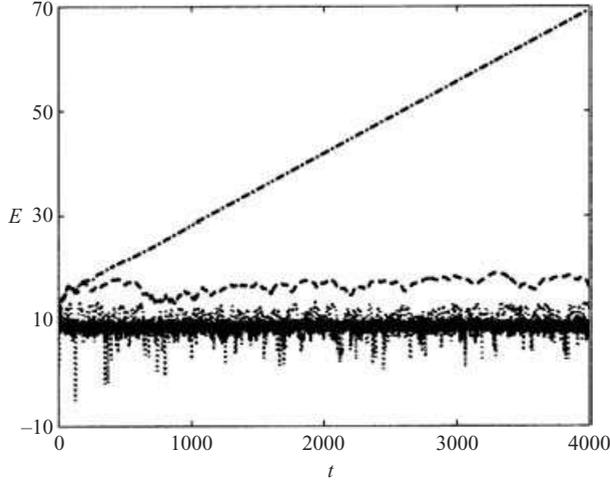
FIGURE 12. Robustness of control scheme with respect to noise: perturbation energy  $E$  as a function of time  $t$  on a semi-log plot for  $\Omega = \Omega_B + 1$ ,  $N = 12$  and  $\ell = 1$ . Random noise of the same energy as the initial condition is added at each time step, with a standard deviation of 36% and spatially distributed over the first  $N$  eigenmodes. Solid line: noise energy; dotted-dashed line: no control; dashed line: with control; dotted line: control energy.
