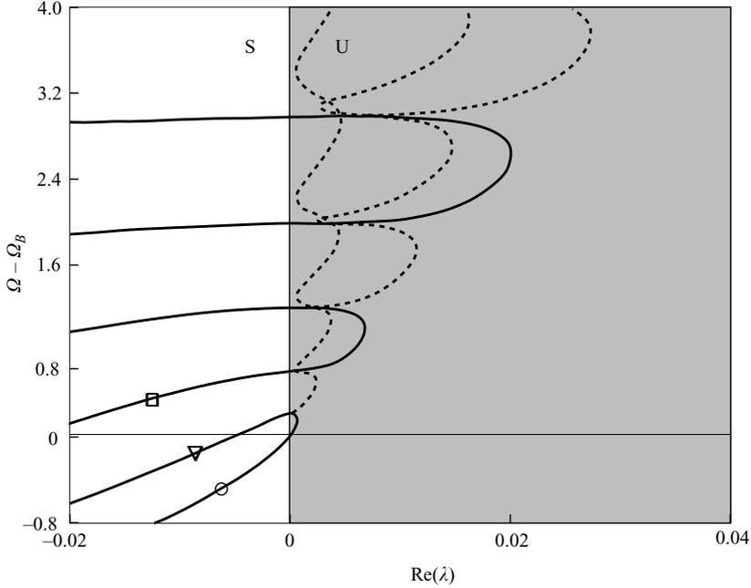
FIGURE 4. Growth rate  $\text{Re}(\lambda)$  of most unstable eigenvalues as a function of swirl parameter  $\Omega - \Omega_B$ . Solid lines refer to real eigenvalues and dashed lines to complex-conjugate pairs of eigenvalues. Symbols on curves refer to eigenvalues plotted in figure 3.
