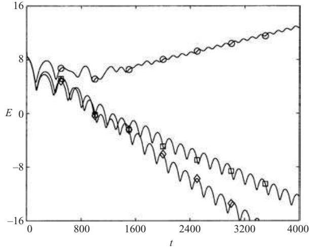
FIGURE 11. Effect of the reduced system order  $N$ . Perturbation energy  $E$  as a function of time  $t$  on a semi-log plot for  $\Omega = \Omega_B + 1.7$ ,  $\ell = 5$  and different values of  $N$ :  $N = 12(\diamond)$ ,  $N = 4(\square)$  and  $N = 3(\circ)$ .
