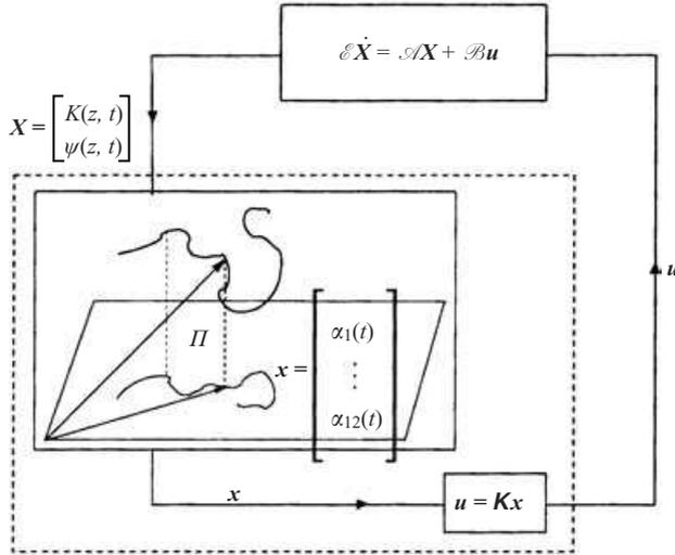
FIGURE 7. Full-state control scheme: the full-state vector  $X$  emerging from the plant is projected on the subspace spanned by the first  $N$  linear eigenmodes by means of the projection operator  $\Pi$ , to yield the reduced-state vector  $x$ . The control given by  $u = Kx$ , where  $K$  is the reduced-order optimal gain matrix, is then fed back into the full plant.
