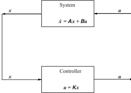
FIGURE 5. Schematic of linear full-information closed-loop control.
