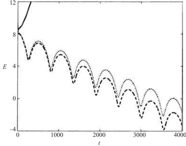
FIGURE 15. Comparison between full-state information control and partial-state information control for  $\Omega = \Omega_B + 1$ ,  $N = 4$  and  $\ell = 1$ : perturbation energy  $E$  as a function of time  $t$  on a semi-log plot. Solid line: no control; dashed line: full-state information control; dotted line: partial-state information control with four sensors.
