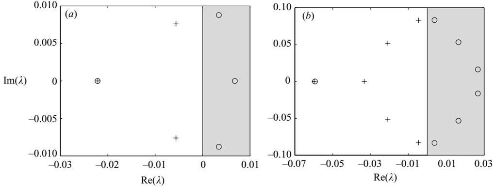
FIGURE 6. Effect of optimal closed-loop control on the most unstable eigenvalues of the reduced-order system;  $\circ$ , eigenvalues without control;  $+$ , eigenvalues with control. (a)  $\Omega = \Omega_B + 1$ ; (b)  $\Omega = \Omega_B + 4$ ; in both cases  $\ell = 1$ .
