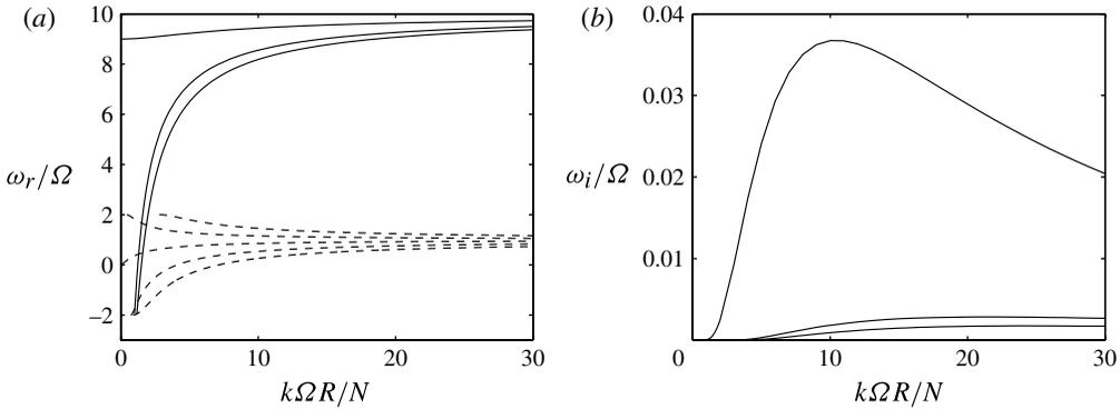
FIGURE 2. (a) Frequency  $\omega_r$  and (b) growth rate  $\omega_i$  as a function of the rescaled vertical wavenumber  $k\Omega R/N$  at  $Ro = -1$ . Dashed lines and solid lines are numerical results for  $m = 1$  and  $m = 10$ , respectively. Only the first three branches are shown.
