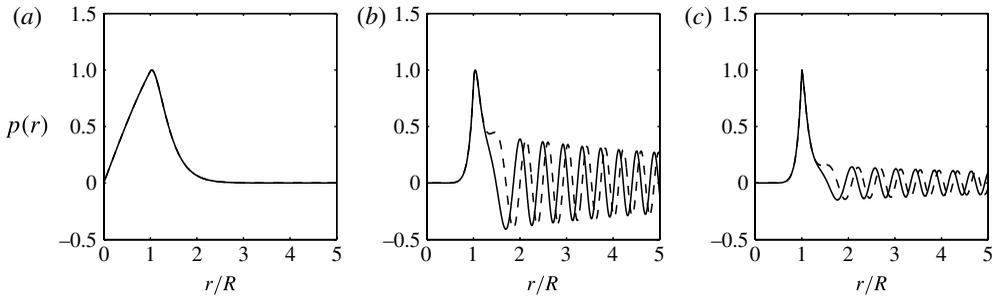
FIGURE 3. Eigenfunctions  $p(r)$  for (a)  $(m, Ro) = (1, -1)$ , (b)  $(m, Ro) = (10, -1)$ , and (c)  $(m, Ro) = (10, -2/3)$  for the first branch at  $kR\Omega/N = 2$ . The solid and dashed lines are the real part and imaginary part, respectively.
