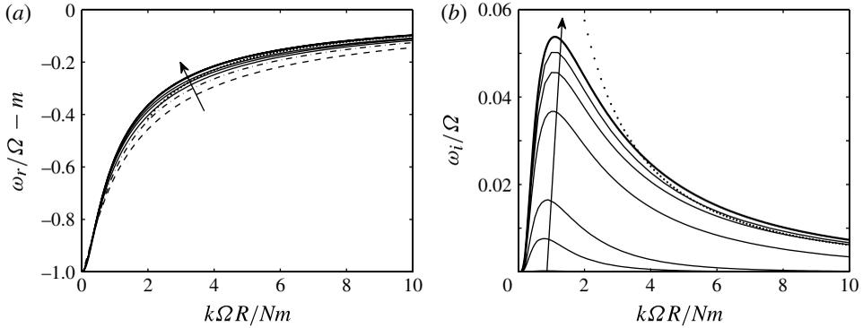
FIGURE 4. (a) Rescaled frequency ( $\omega_r/\Omega - m$ ) and (b) growth rate  $\omega_i$  as a function of rescaled vertical wavenumber  $k\Omega R/(Nm)$  at  $Ro = -1$ . The dashed line, dot-dashed line and solid lines are numerical results for  $m = 1, m = 2$  and  $m = [3, 4, 5, 10, 20, 50]$ . The arrows indicate an increase of  $m$ . The bold and dotted lines are asymptotic results for large  $m$  (4.2) and for both large  $\tilde{k}$  and  $m$  (A 6) for  $m = 20$ , respectively.
