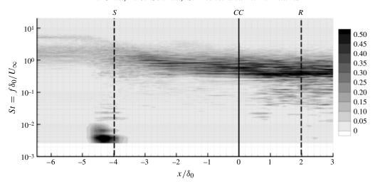
FIGURE 6. Contours of the weighted power spectral density of wall pressure in the  $St-x/\delta_0$ -plane. The power spectral density is normalized such that their integral over frequency is unity. Thirty contours levels have been used; the dashed vertical lines indicate the location of the separation S and reattachment point R respectively. The solid line indicates the position of the corner CC.
