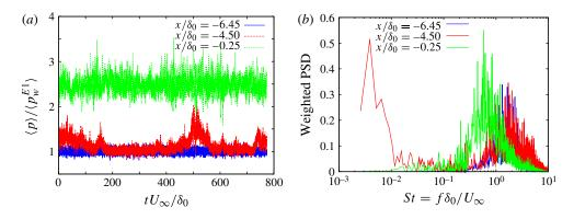
FIGURE 5. (a) Wall-pressure signals and (b) corresponding weighted power spectral density at different streamwise locations relative to the ramp corner.
