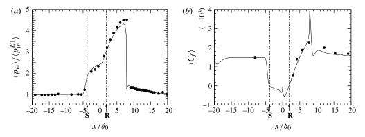
FIGURE 4. Averaged wall-pressure (a) and skin-friction coefficient (b) distributions versus the streamwise direction. The symbols indicate the reference experiment, the solid line represent results from the LES, averaged in time and over the spanwise direction. The labels S and **R** mark the mean separation and reattachment point, respectively.
