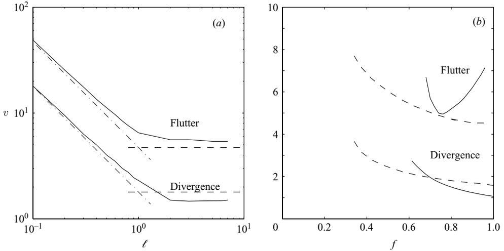
FIGURE 8. Model of the stability of a long cylinder using the stability diagram of a short cylinder of effective length  $\ell = 1$ . (a) Effect of length on the critical velocities for divergence and flutter for  $f = 0.8$ ; —, present results; ---, short cylinder approximation, equation (5.1); -.-, long cylinder approximation, equation (5.2). (b) Stability diagram: -.-, long cylinder approximation (5.2) for divergence and for flutter compared to the present results for long cylinders (—).
