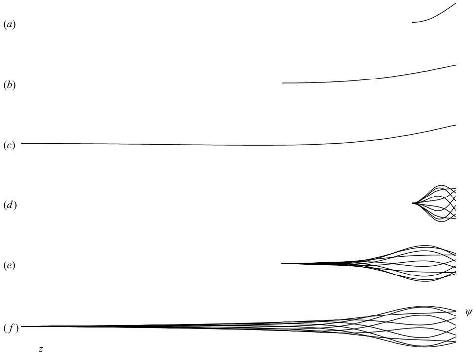
FIGURE 4. Modal shape  $\psi(z)$  of the unstable modes as a function of the length of the cylinder for  $f = 0.8$ . (a–c) Divergence mode shape for  $\ell = 0.5, 2, 5$ , respectively. (d–f) Flutter motion over a cycle of oscillations reconstructed from the complex mode shape at  $v = 1.1v_F$  for  $\ell = 0.5, 2, 5$ , respectively.
