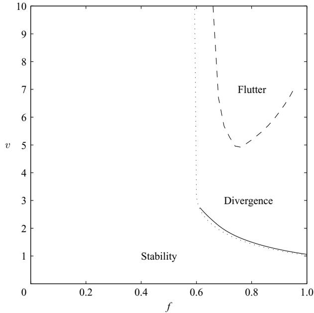
FIGURE 6. Stability diagram for long cylinders,  $\ell \gg 1$ , from computations at  $\ell = 10$ , depending on the parameter  $f$  relative to the shape of the downstream end. —, Divergence limit; ---, flutter limit;  $\dots$ , exact divergence limit adapted from the solution of Triantafyllou & Chryssostomidis (1984), using (4.2) with the change of variables of (4.3).
