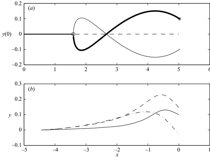
FIGURE 5. Solution of the nonlinear equation of motion for a long cylinder,  $\ell = 4.44$ ,  $f = 0.8$ . (a) Bifurcation diagram of the displacement at the downstream end when the flow velocity is varied. o, Divergence at  $v = 1.59$ ; \*, flutter at  $v = 5.03$ . (b) Deformation of the cylinder for three flow velocities along the branch in bold line:  $-\cdot-$ ,  $v = 2.5$ ;  $---$ ,  $v = 3.5$ ;  $—$ ,  $v = 5$ .
