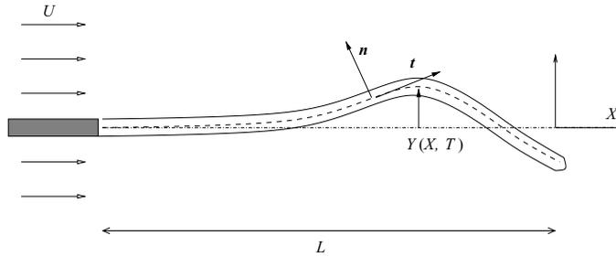
FIGURE 1. A long cantilevered cylinder in axial flow.
