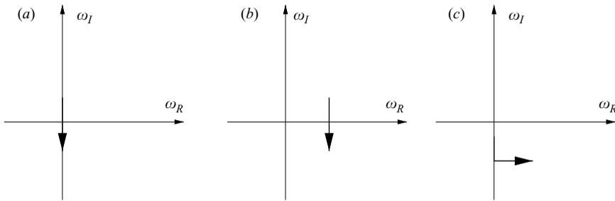
FIGURE 2. Types of instability, depending on the crossing of axes in the complex  $\omega$ -plane. (a) Divergence, (b) flutter by Hopf bifurcation, (c) flutter of the Païdoussis type.
