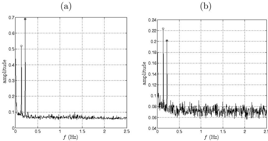
**Figure 5.** Spectrum associated with the DMD  $\alpha_k$  of the spanwise dataset
