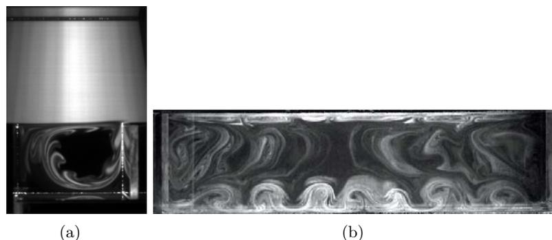
**Figure 2.** Smoke visualization for a cavity geometry  $L/H = 1.5$ ,  $S/H = 6$  and for a typical Reynolds number  $\Re_H \approx 3000$ . (a) Front view of the longitudinal plane  $(x, y)$ , (b) top view of the spanwise plane  $(x, z)$  located at  $y/H = -0.3$  inside the cavity.
