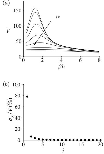
Figure 3: (a) Dependence of the variance  $V$  of the response to stochastic forcing on the dimensionless spanwise wavenumber  $\beta h$  for selected streamwise wavenumbers  $\alpha$  (same values as in Fig. 2: top to bottom  $\alpha h = 0, 0.1, 0.25, 0.5, 1, 2, 3, 4$ ). (b) Contribution of the leading 20 Karhunen-Loëve modes to the total variance.
