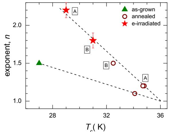
FIG. 4. (Color online) The exponent  $n$  of the power-law fit of  $\Delta\lambda(T)$  from Fig. 3, vs  $T_c$ . Note the significantly smaller exponents for as-grown and annealed compared to the samples with irradiation defects. The dashed lines are guides for the eye.
