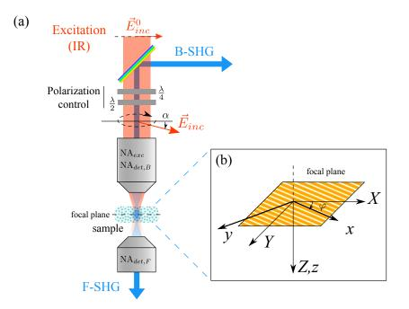
Fig. 1. (a) Setup geometry. Excitation polarization angle  $\alpha$  is controlled by two achromatic waveplates. Excitation field  $\vec{E}_{inc}$  is then focused through an objective  $(NA_{exc})$ . SH radiation is collected forwards with a condensor  $(NA_{det,F})$  and backwards through the focusing objective  $(NA_{et,B} = NA_{exc})$ . (b) Zoom in the focal plane. (XYZ) is the laboratory frame, (xyz) is the fibril frame with *x* the fibril axis.
