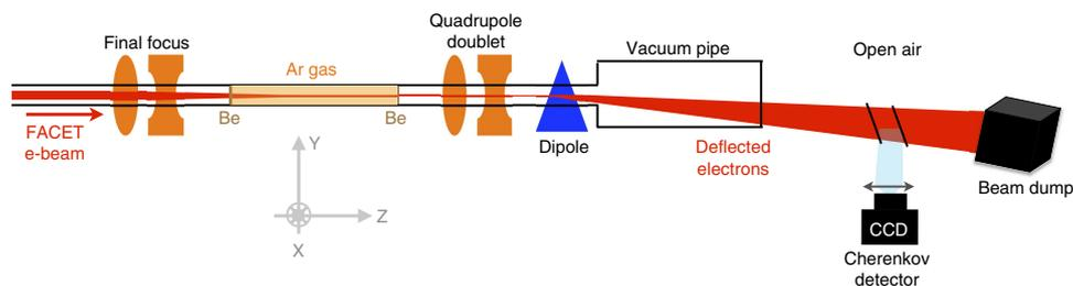
**Figure 1 | Schematic diagram of the experimental setup.** The FACET electron beam is focused by final focus quadrupoles inside a volume filled with argon gas and contained by two beryllium windows. After interacting with the plasma, electrons are transported by a quadrupole doublet towards the beam dump and deflected vertically by a dipole magnet. A Cherenkov detector is used to measure the electron energy spectrum (see the Methods for details).
