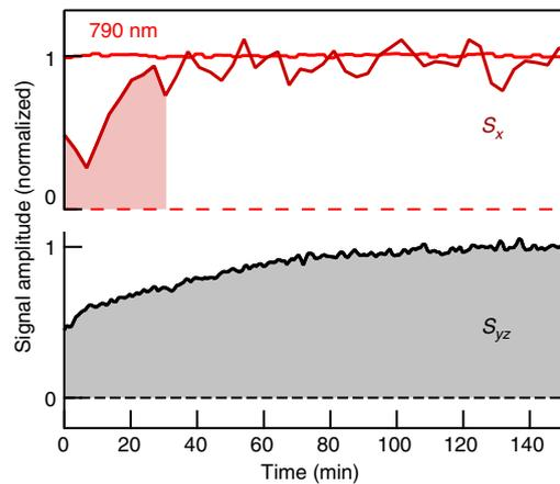
**Figure 2 | Long-term signal changes.** Evolution of the amplitudes of THz signals  $S_x$  and  $S_{yz}$  and the reflectance of the 790 nm pump beam following cleaving of the sample. The constant 790 nm signal indicates that no sample damage occurs.
