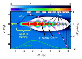
Figure 4 | Reconstruction of the longitudinal variation of  $\emph{F}_{\emph{z}} = -\,\emph{eE}_{\emph{z}}.$
