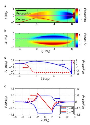
Figure 1 | From simulation: distribution of forces within the cavity.
