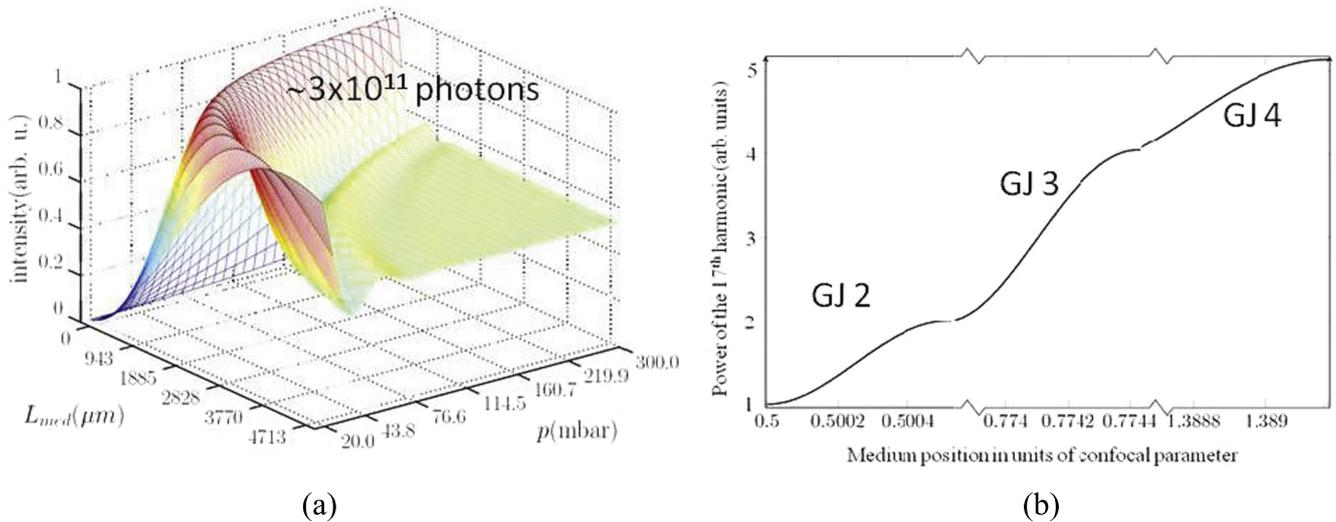
**Figure 17.** (a) Numerical simulations of the atomic response and phase matching in one argon jet showing the photon number of the 17<sup>th</sup> harmonic as a function of the argon gas length and pressure. The laser parameters are: pulse duration  $\approx 5$  fs, energy  $\approx 100$  mJ/pulse, carrier wavelength  $\approx 800$  nm and the focal length 10 m. (b) Demonstration of the 17<sup>th</sup> harmonic energy enhancement by additional gas jets (GJ 2–4) with argon gas at 50 mbar.
