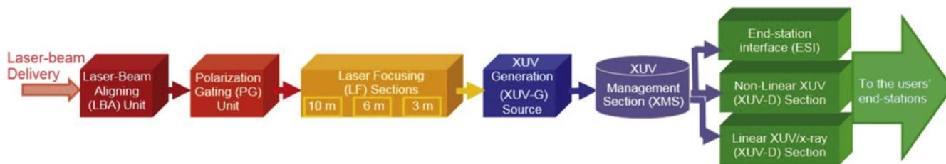
**Figure 13.** Block diagram of the SYLOS-driven users HHG beamline. The beamline consists of LBA, collinear waveplate PG, LF supporting three different focal lengths, XUV-G based on a gaseous non-linear medium, XUV-BS, steering and spectral-range-selecting section (XMS), XUV-D with subsections for XUV-CC and XUV-AC measurements, as well as a number of other diagnostics, and the end station interfacing (ESI) branch.
