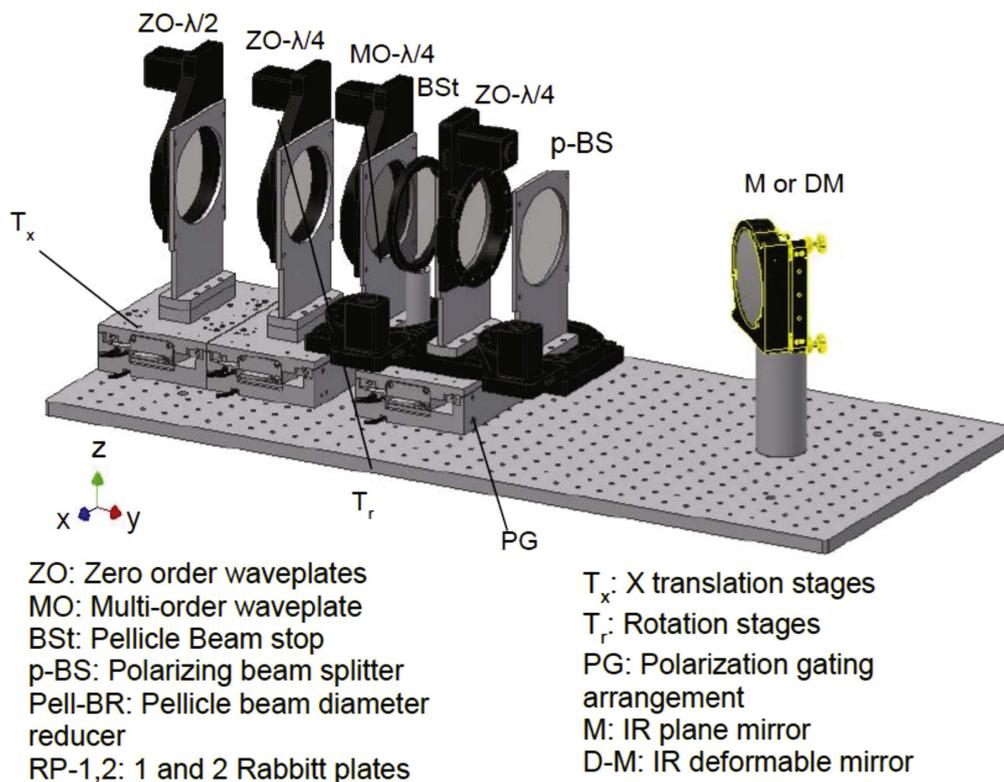
**Figure 18.** Polarization control and gating setup (PG2 chamber).
