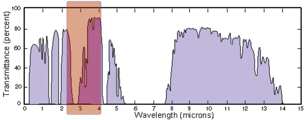
Figure 4. Atmospheric transmittance and the MIR laser emission band.
