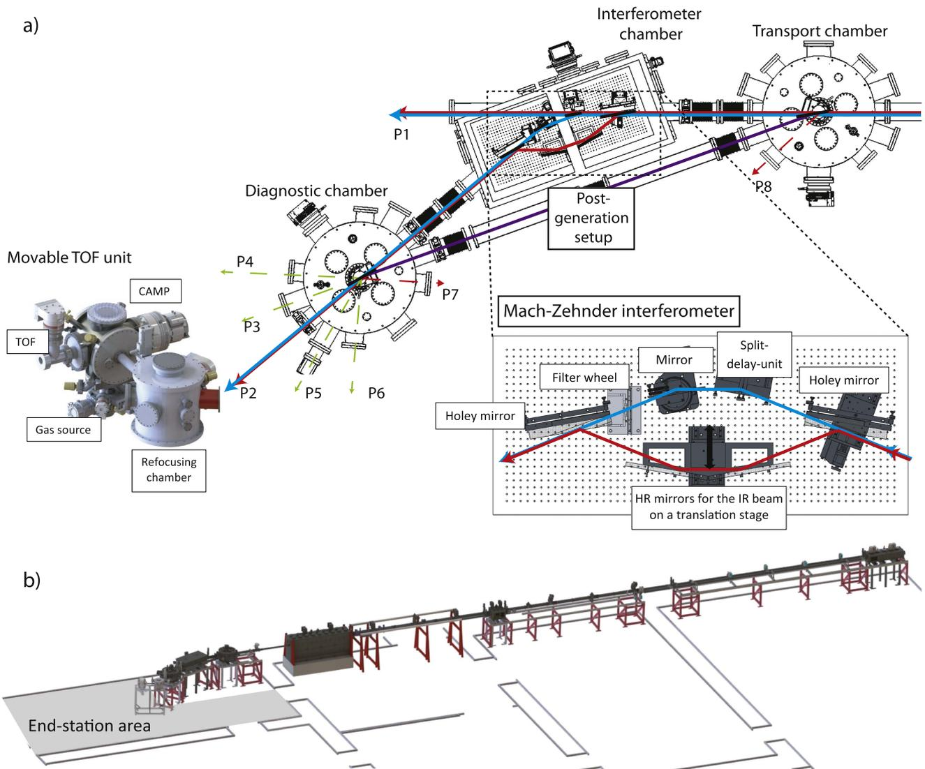
**Figure 23.** (a) The pump-probe setup: Mach-Zehnder interferometer with a split-delay-unit and additional arm (the violet beam path) for post-generation setups; (b) 3D view of the beamline with indicated space for dedicated and user end stations.
