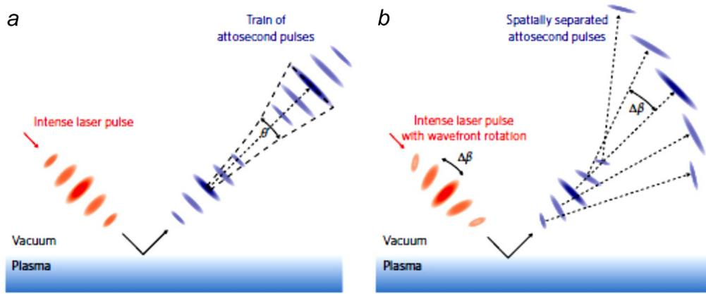
**Figure 28.** The basic principle of the attosecond lighthouse. (a) Attosecond pulse train from pulses without wavefront rotation. (b) Attosecond pulse train from pulses with wavefront rotation. [94] (2017) Figure reprinted with permission of Springer.
