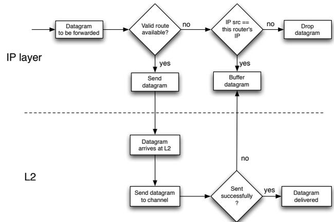
Figure 1. Link buffering process for L3 and L2
