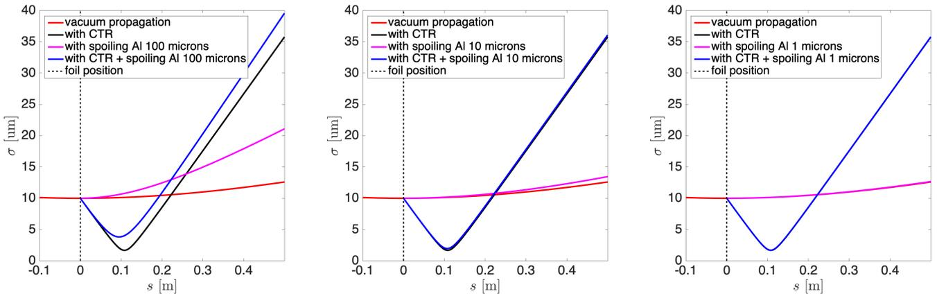
Figure 3: **Beam evolution with multiple scattering included and  $3 \mu\text{m}$  normalized emittance.** Evolution of the beam size with the propagation distance with and without foil, for an initial waist located at the foil position and for a beam size of  $10 \mu\text{m}$  at the waist. The effect of multiple scattering is taken into account for an aluminum foil with a thickness of  $100 \mu\text{m}$  (left),  $10 \mu\text{m}$  (middle) and  $1 \mu\text{m}$  (right).
