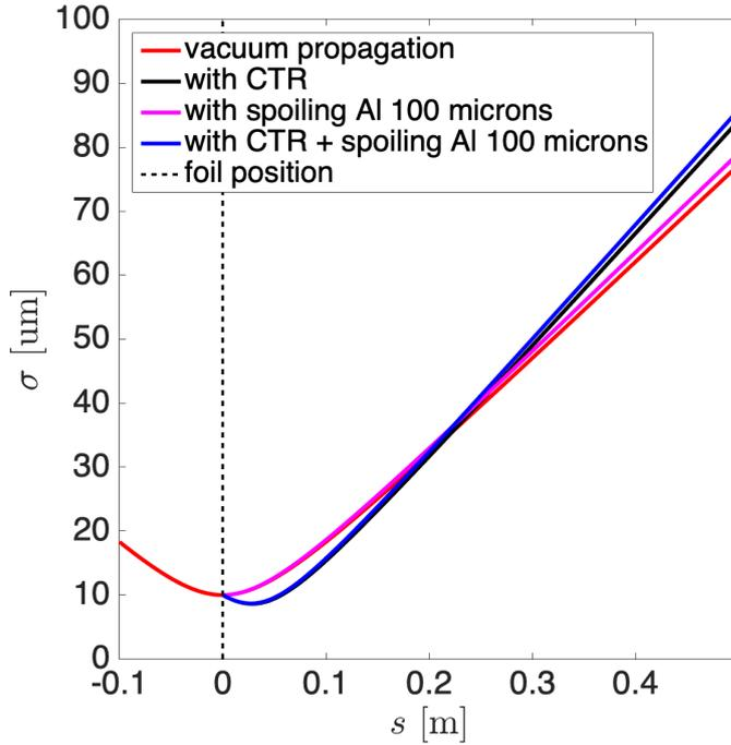
Figure 2: **Beam evolution with multiple scattering included and  $30 \mu\text{m}$  normalized emittance.** Evolution of the beam size with the propagation distance with and without foil, for an initial waist located at the foil position and for a beam size of  $10 \mu\text{m}$  at the waist. The effect of multiple scattering is taken into account for an aluminum foil of  $100 \mu\text{m}$  thickness.
