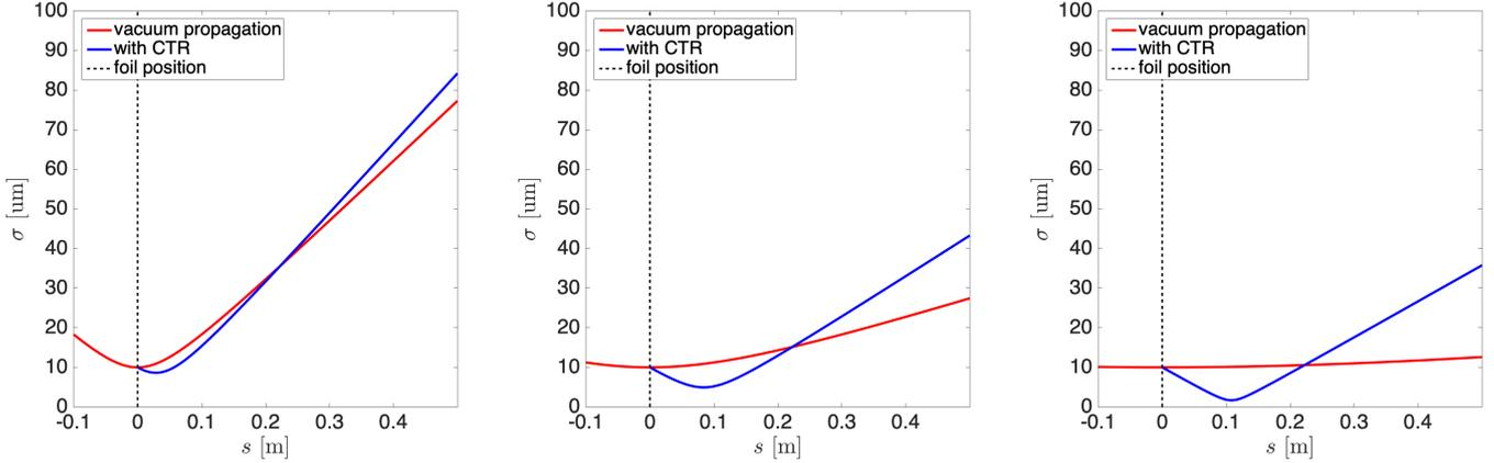
Figure 1: **Beam evolution and focusing effect from near-field transition radiation.** Evolution of the beam size with the propagation distance with and without foil, for normalized emittances of 30  $\mu\text{m}$  (left), 10  $\mu\text{m}$  (middle) and 3  $\mu\text{m}$  (right), and for an initial waist located at the foil position and for a beam size of 10  $\mu\text{m}$  at the waist. The effect of multiple scattering is not taken into account.
