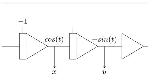
■ **Figure 2** Example of GPAC circuit: computing sine and cosine with two variables.
