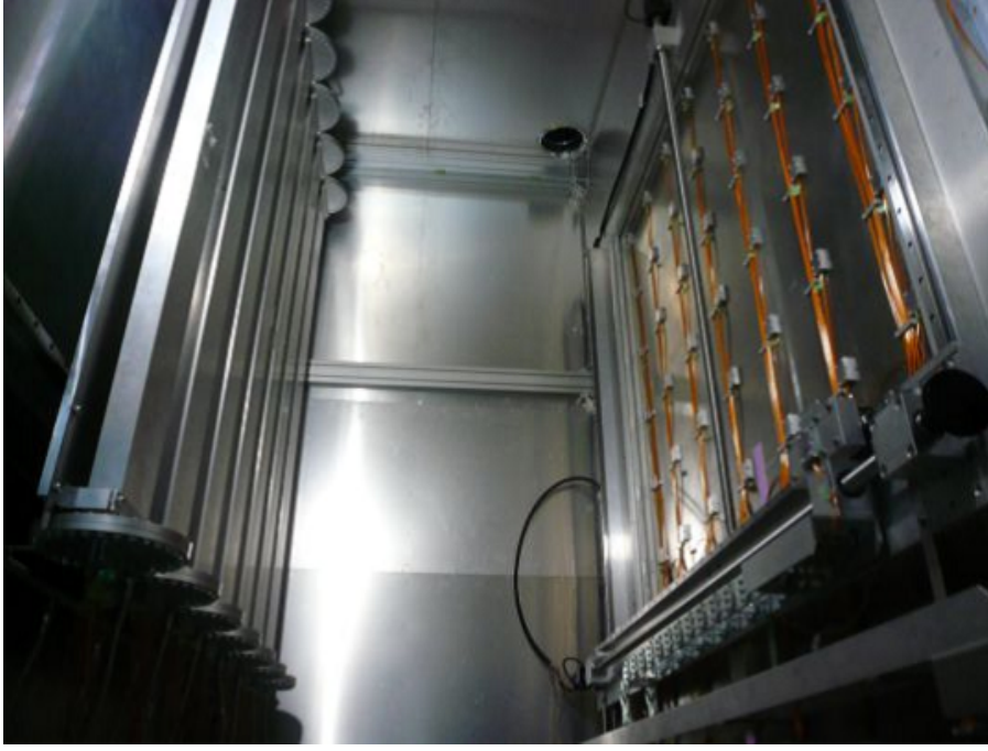
Figure 2.12: The muon monitor (MuMon). The ionisation chamber is shown on the left and the PIN photodiodes-based detector on the right. The muon and neutrino beams go from the left to the right.
