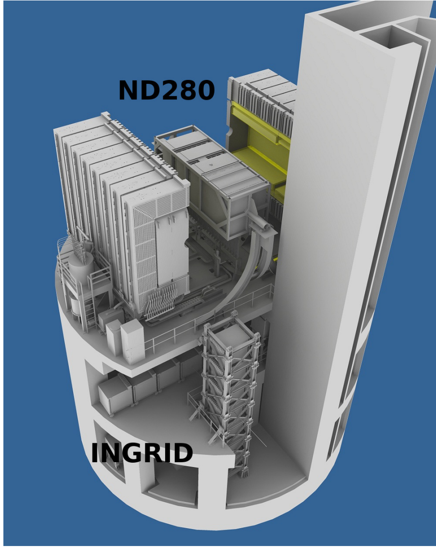
Figure 2.13: The T2K near detector complex. The INGRID vertical and horizontal modules can be seen on the bottom part. The ND280 off-axis detector is visible on the top part with its magnet open.
